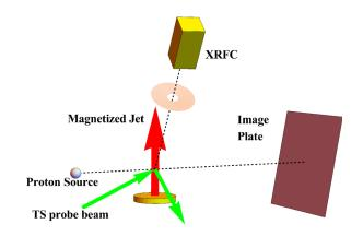
**FIG. 2.** Schematics of the diagnostics setup of OMEGA magnetized jet experiments. For DD and D $^3$ He protons, the source stands 1 cm from TCC, while the image plate CR39 is located 17 cm from TCC on the other side. For the TNSA protons, the source stands 0.8 cm from TCC, while the radiochromic film pack is located 16.5 cm from TCC on the other size. The X-ray framing camera (XRFC) images the jet at 38° from the axis, which is not modeled in this work.
