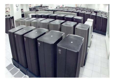
a distributed memory computer with 6,080 processors. Each processor has a peak performance of 1.5 GFlops. The processors are distributed among 380 compute *nodes* with 16 processors per node. Processors on each node have a shared memory pool of between 16 and 64 GBytes
