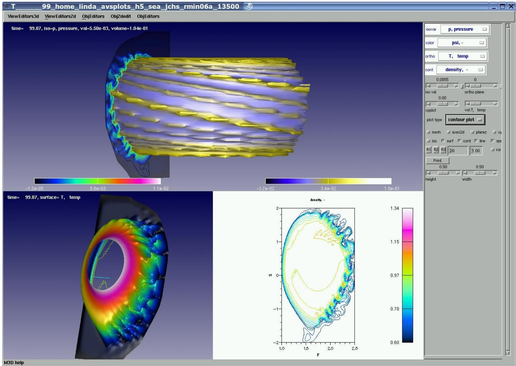
t=492. Long time saturation - healing to near original configuration. Perturbation at plasma edge develops on dominant field lines.
