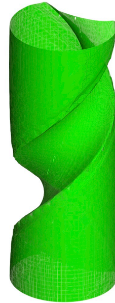
Isosurfaces of density from a nonlinear external kink computation.
