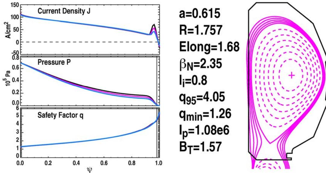
Figure 1. The profiles of current density, pressure and  $q$  for three equilibria used in this study, some common parameters for one of these equilibria, and the shape of one of these equilibria. The parameter values and shape do not change significantly between the three cases.
