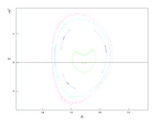
Lack of poloidal resolution (my = 16 with cubic polynomials) unable to resolve pressure flattening inside 3/2 island.
