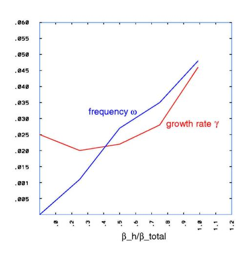
circular tokamak R/a=2.76 q(0)=0.6, q(a)=2.4  $\beta$ \_total(0) = 8%  $v_h/v_A$  = 1.0,  $\rho_h/a$ =0.05 Isotropic slowing-down hot particle distribution
