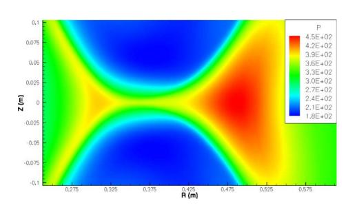
Pressure profile near the reconnection site from a simulated counter-helicity push configuration.
