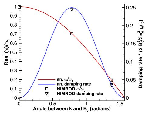
$\text{ The analytical dispersion relation is } \omega^2 + \left(\omega_0^2 \frac{k_{||}^2}{k^2}\right) \left(i\frac{3\eta_0\mu_0k_\perp^2}{B_0^2k^2}\omega - 1\right) = 0 \text{ , } \omega_0^2 \equiv \Omega_i^2d_i^4k^4$  and for weak damping,  $\omega_r^2 \cong \omega_0^2 \frac{k_{||}^2}{k^2} \quad , \quad \omega_i \cong -\omega_0^2 \left(\frac{3\eta_0\mu_0k_{||}^2k_\perp^2}{2B_0^2k^4}\right)$
