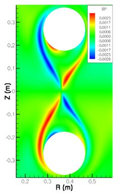
Out-of-plane component of magnetic field induced by Hall effect during simulated pull reconnection without guide field.
