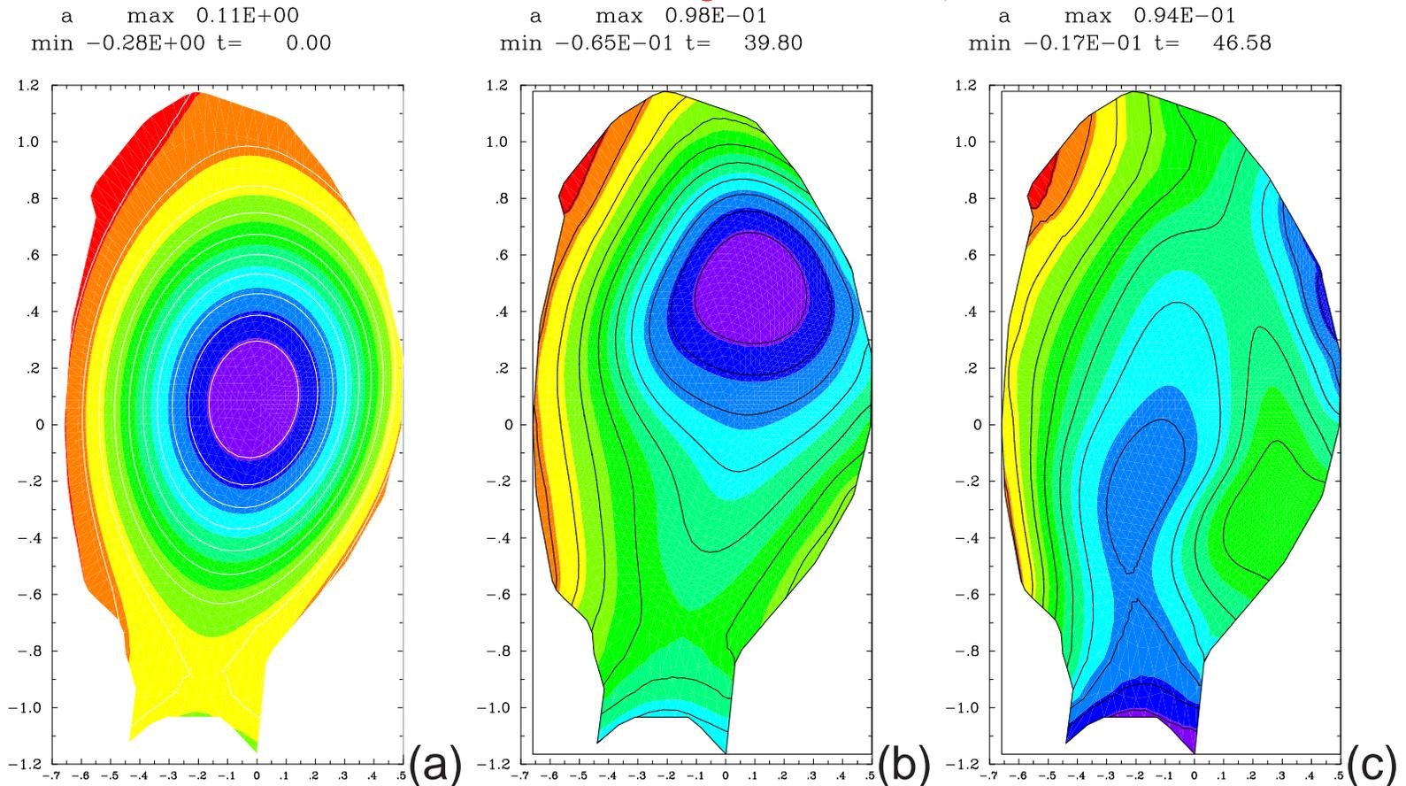
(a) initial magnetic flux contours of rescaled ASDEX equilibrium reconstruction. (b) magnetic flux contours in the poloidal plane with toroidal angle  $\phi = 0$ , at time  $t = 39.8\tau_A$ . The flux resembles a typical VDE. (c) magnetic flux contours in the poloidal plane with toroidal angle  $\phi \neq 0$ , at time  $t = 46.6\tau_A$ . There are no closed poloidal flux contours.
