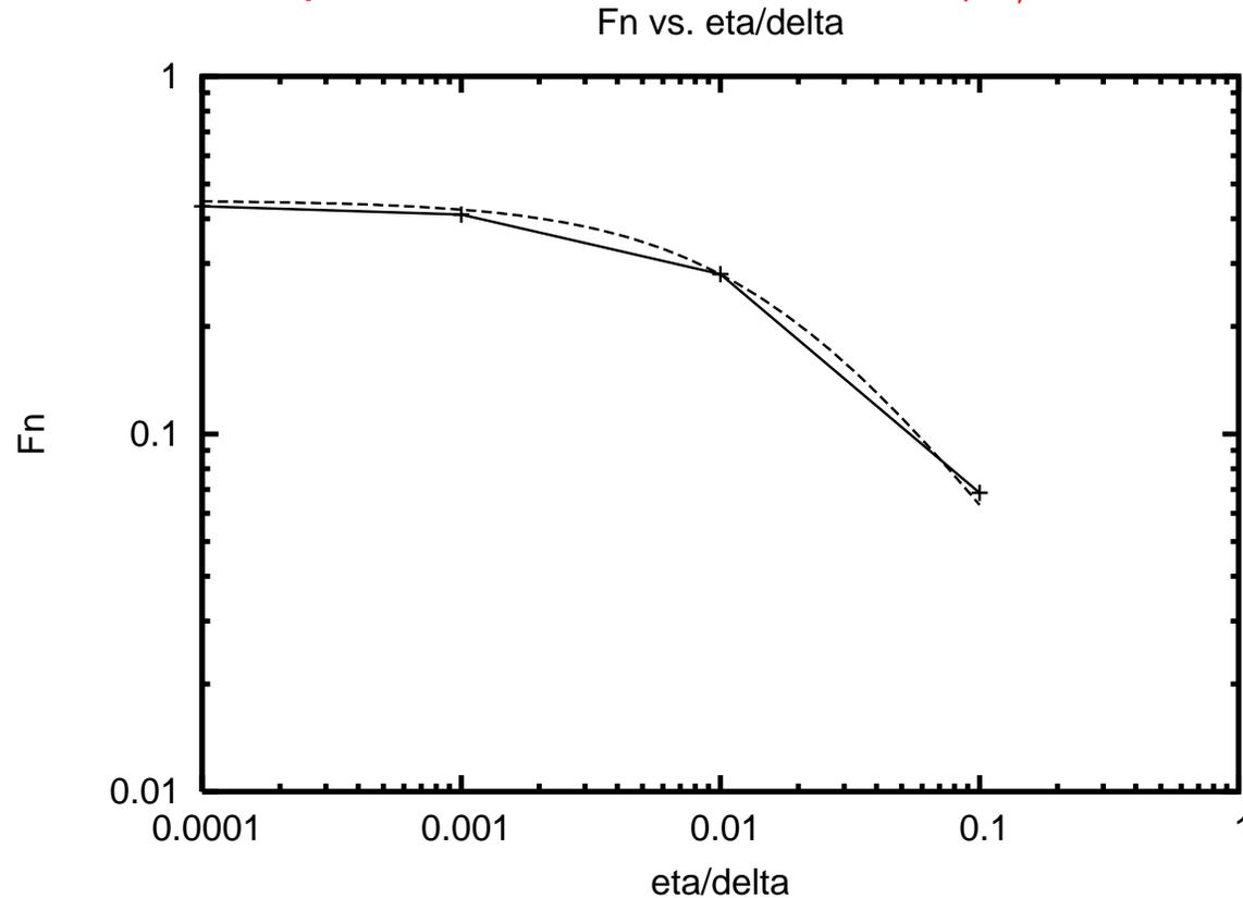
Variation of peak wall pressure  $P_w = F_w n \delta / B_0^2$  as a function of wall resistivity divided by wall thickness,  $\eta_w/\delta$ . The data is well fit by the formula,  $P_w \propto 1/(1 + \alpha \eta_w/\delta)$  where  $\alpha = 0.0125$ .
