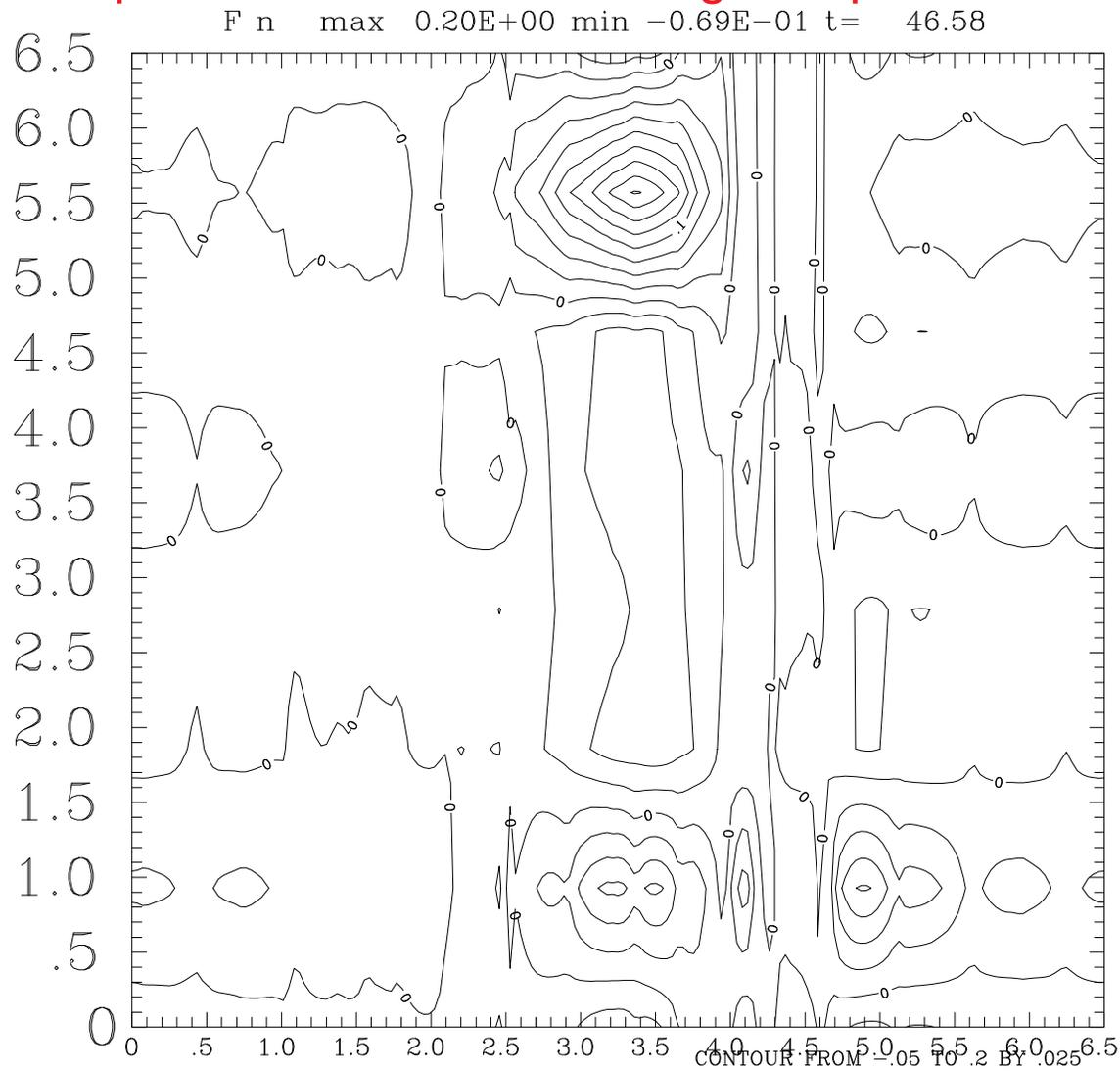
magnetic pressure on the wall as a function of poloidal angle (horizontal) and toroidal angle (vertical) at time  $t = 46.6\tau_A$ .
