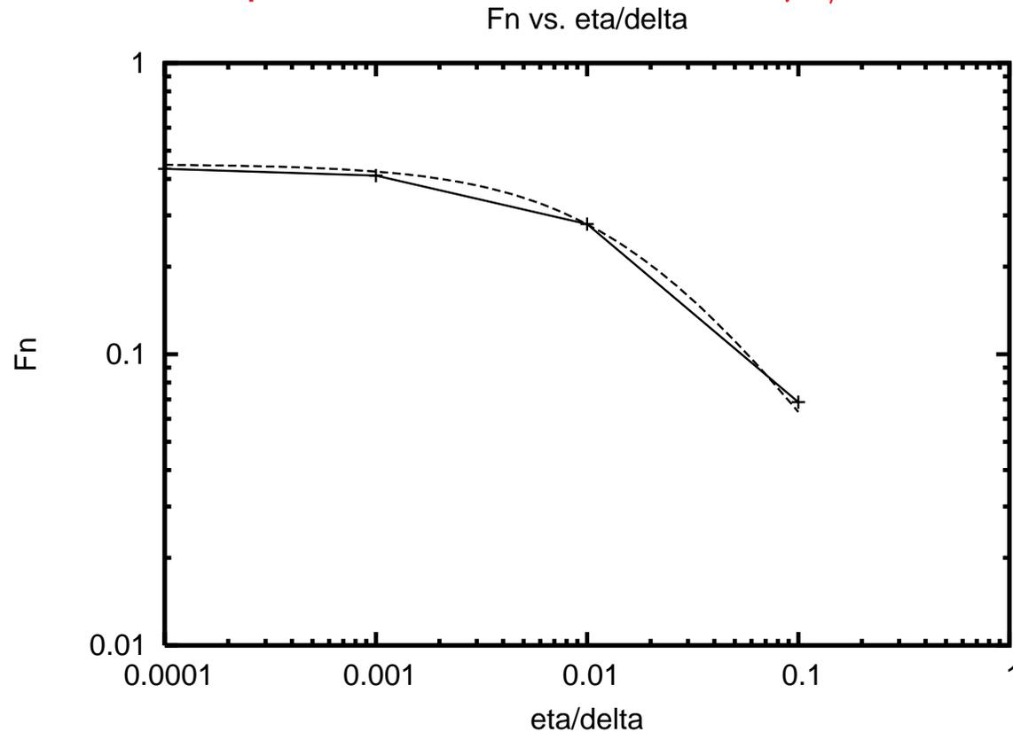
Variation of peak wall pressure  $P_w = F_w \eta_w \delta / B_0^2$  as a function of wall resistivity divided by wall thickness,  $\eta_w/\delta$ . The data is well fit by the formula,  $P_w \propto 1/(1 + \alpha \eta_w/\delta)$  where  $\alpha = 0.0125$ .
