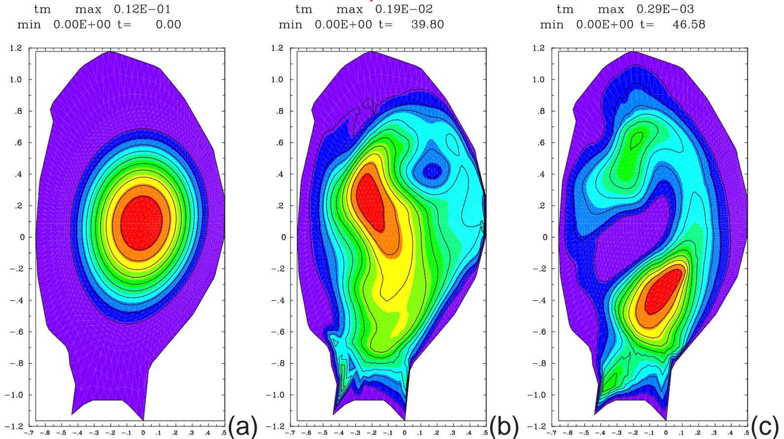
(a) initial temperature contours in the poloidal plane with toroidal angle  $\phi = 0$ . (b) temperature contours at  $t = 39.8\tau_A$ . The temperature has dropped a factor of 6 from its initial peak. (c) temperature contours at time  $t = 46.6\tau_A$ , where the temperature has dropped by a factor of 40 from the initial peak.
