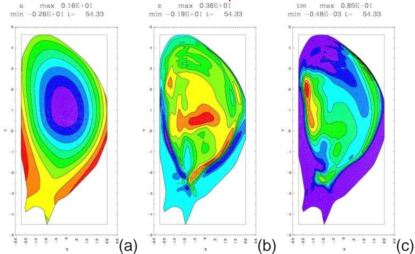
(a) poloidal flux  $\psi$ , (b) toroidal current  $-RJ_\phi$ , (c) temperature  $T$ , at  $t = 54.3\tau_A$ , with toroidal angle  $\phi = \pi$ . Current sheet, current and temperature maxima penetrate the wall.
