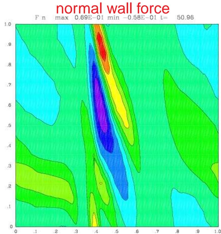
normal force density at  $t = 51\tau_A$ ,  $f_n(\theta, \phi)$ , where  $\theta$ , the poloidal angle from the origin, is the horizontal axis.
