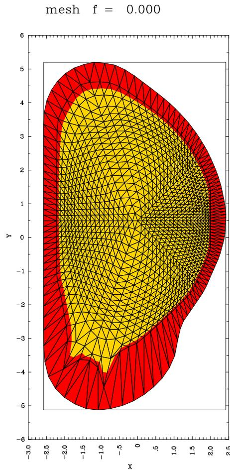
ITER has two walls.  $\tau_w^{outer} \gg \tau_w^{inner}$ . M3D modeling assumes  $\tau_w^{inner} = 0$ . The magnetic field is continuous at inner wall, no force on inner wall. Forces on outer wall are about 25 % of forces in one wall model. Simulation results of 2 wall and 1 models are qualitatively similar.
