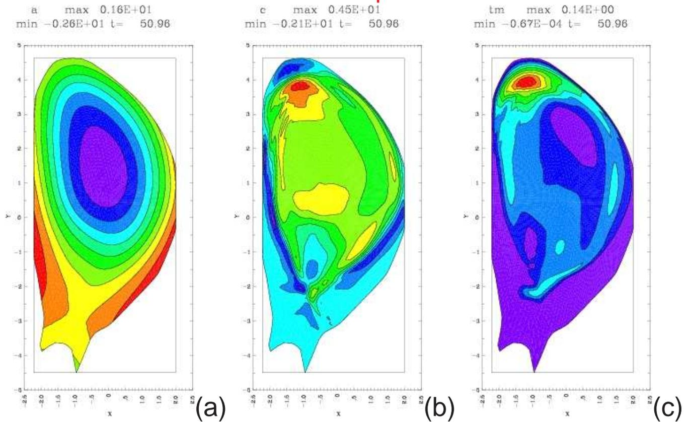
(a) poloidal flux  $\psi$ , (b) toroidal current  $-RJ_\phi$ , (c) temperature  $T$ , at  $t = 51\tau_A$ , with toroidal angle  $\phi = \pi$ .
