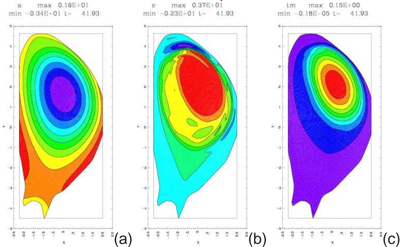
(a) poloidal flux  $\psi$ , (b) toroidal current  $-RJ_\phi$ , (c) temperature  $T$ , at  $t = 40.9\tau_A$ , with toroidal angle  $\phi = \pi$ . This example has  $I/I_0 = 2$ , and  $\gamma\tau_w \approx 15$ . A VDE brings the plasma to the upper wall, where an  $(m, n) = (1, 1)$  kink mode grows.
