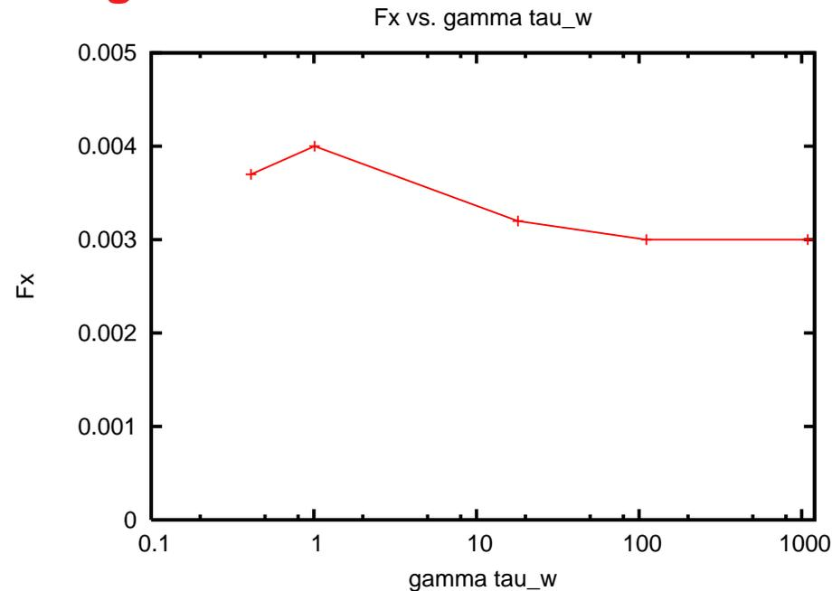
Scaling of horizontal  $F_x$ , with  $\gamma\tau_w$ . The cases shown have  $I/I_0 = 1.6$ . The force tends to a limit for an ideal conducting wall  $\gamma\tau_w = \infty$ . Flux penetration is important for  $\gamma\tau_w = 1$ .
