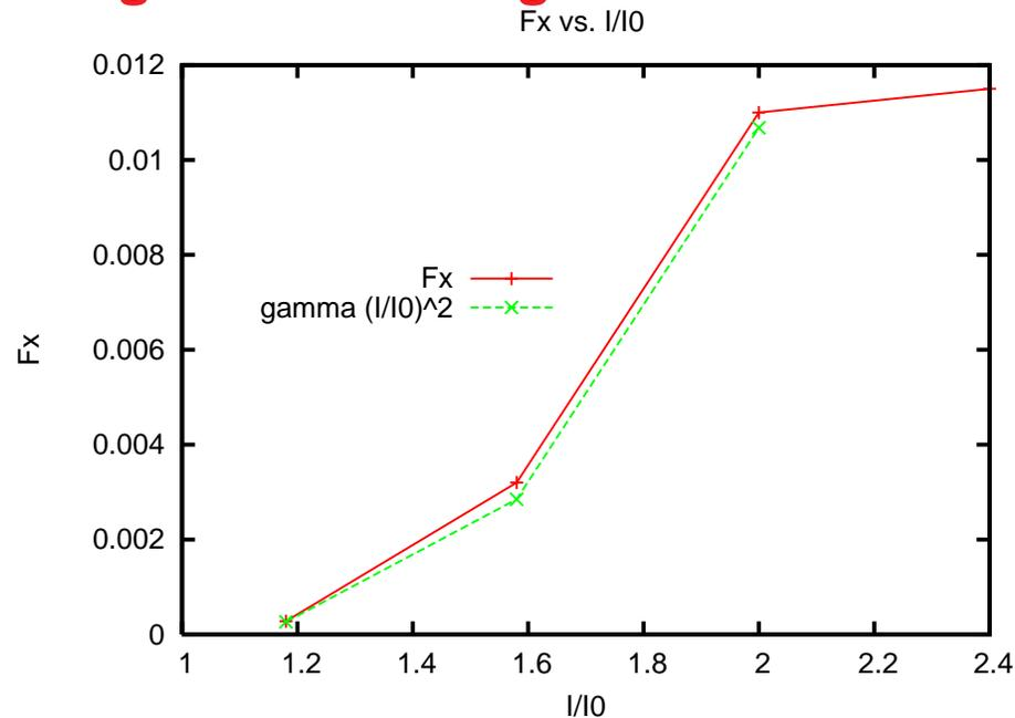
Scaling of wall averaged non axisymmetric horizontal force density with total current  $I/I_0$ . Fit is  $\propto \gamma(I/I_0)^2$ . This scaling fits for  $I/I_0 \leq 2$ , and saturates for larger  $I/I_0$ . The horizontal force is as large as 1.2 % of the total magnetic pressure.
