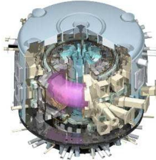
Disruptions have become an ITER issue. They can cause large electromechanical stress on conducting structures. ITER wall forces can be more than 10 times larger than in existing tokamaks. Need more info on worst case scenario, avoidance, mitigation. Main concern is “sideways force.”
