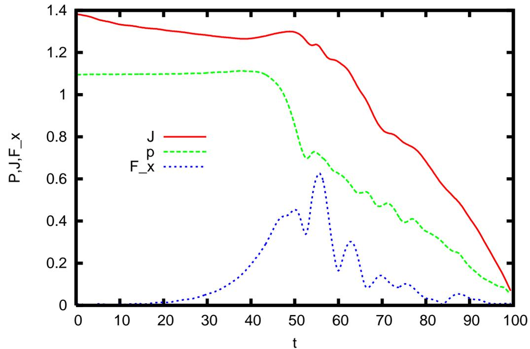
total toroidal current  $I_\phi$ , total pressure  $P$ , TPF, and horizontal force  $F_x$  as a function of time, in arbitrary units.
