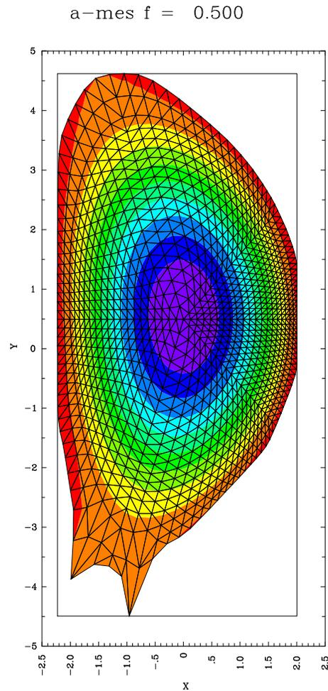
Simulations are done with the M3D code used at PPPL, a 3D initial value resistive MHD code. Unstructured mesh (Strauss and Longcope, 1988) shown at low resolution, in poloidal (R,Z) plane and pseudospectral (Fourier) representation in toroidal  $\phi$  direction. Upwinding and dealiasing provided adequate numerical stabilization to permit the simulation of complete disruption events. The open field line "vacuum" region surrounding the plasma is modeled with high resistivity.
