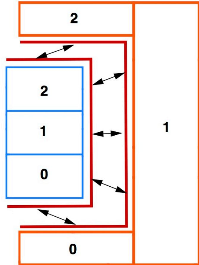
**Schematic shows a 2-region, 3-process example. Each region has subdomains, and processes are numbered from 0.**
