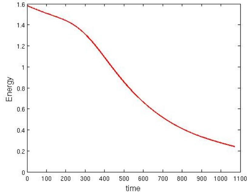
**Internal energy decays faster than current after  $300 \tau_A$  due to thermal transport from outer surfaces.**
