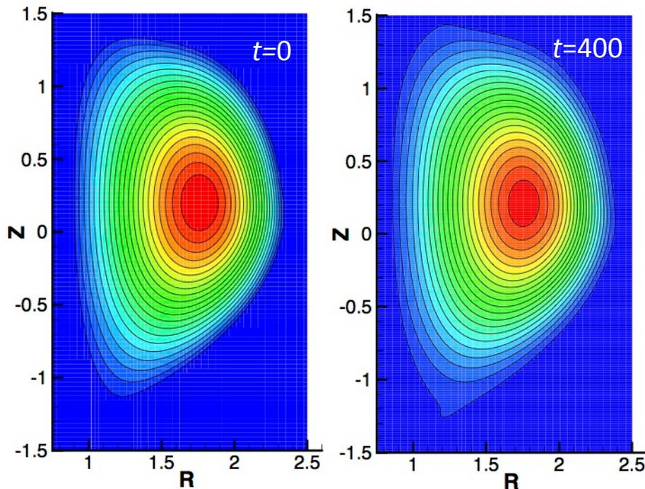
Comparison of initial and final  $T$  profiles indicates slight spreading near separatrix.
