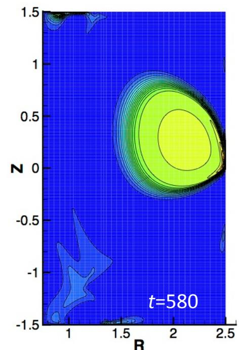
The evolution of current and thermal energy is essentially unchanged when the normal component of flow is set by  $\mathbf{E}_w \times \mathbf{B}$  drift.
