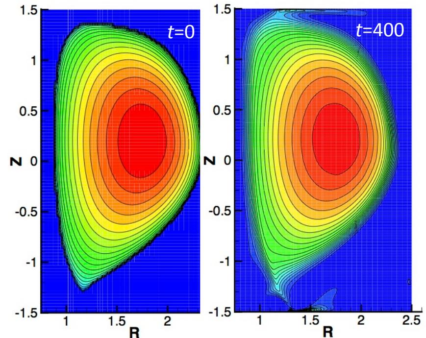
Comparison of initial and final  $n$  profiles shows weak diffusion and some leakage.
