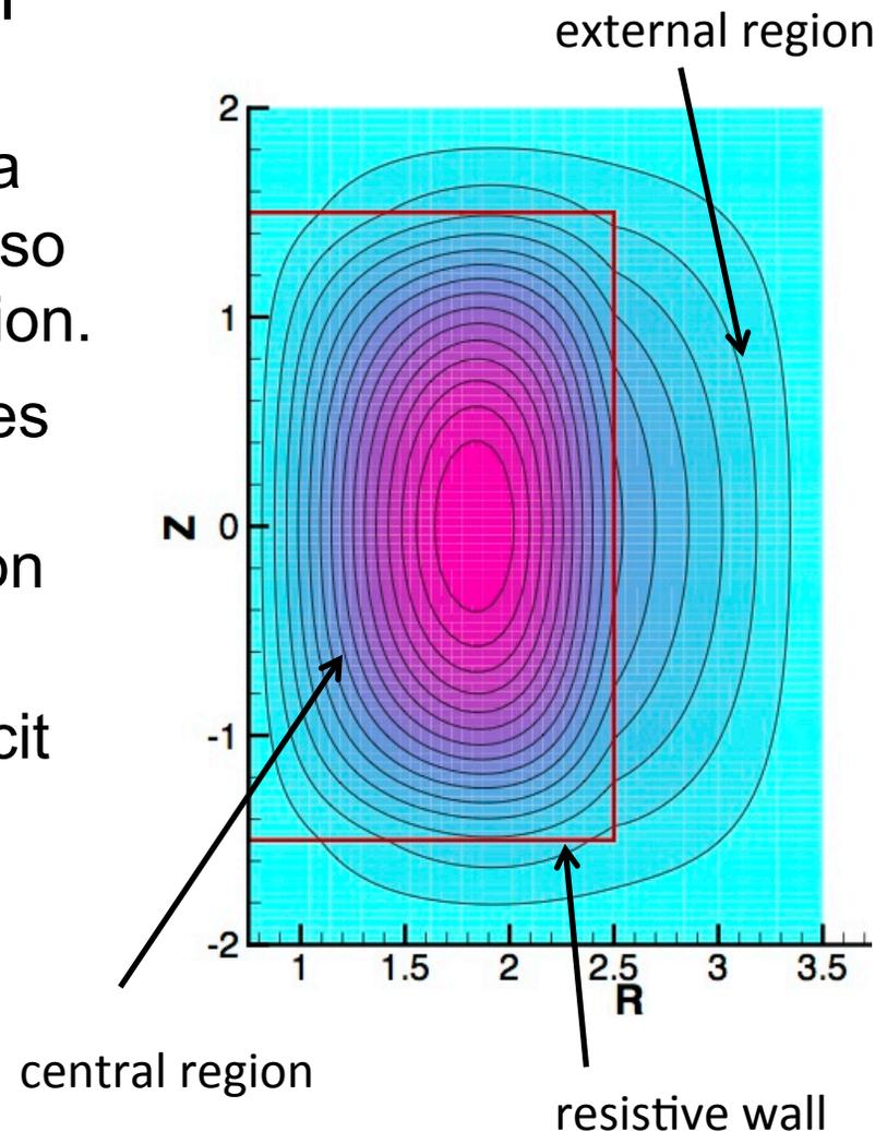
Boundary conditions on  $\mathbf{B}$  are set at the outer boundary, while conditions on  $n$ ,  $T$ , and  $\mathbf{V}$  are set along the perimeter of the central region.
