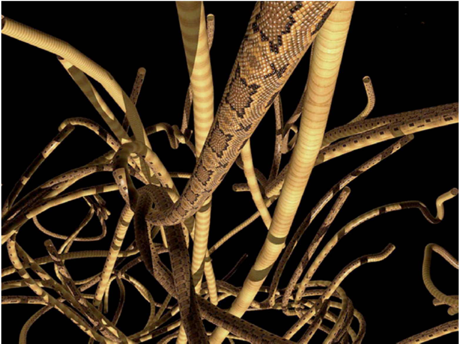
Fig. 3. 3-D currents of Alfvén waves in a helium plasma rendered as snakes using the graphics package “Maya.” For this image, the background magnetic field points out of the page. This image is part of a sequence used in the creation of a 3-D movie in collaboration with Eric de Jong, Steve Levoe, and Shigeru Suzuki from the Jet Propulsion laboratory, Pasadena, CA. The movie was shown in a lecture at the Los Angeles County Museum of Art and demonstrates (if nothing else) a link between science and art.
