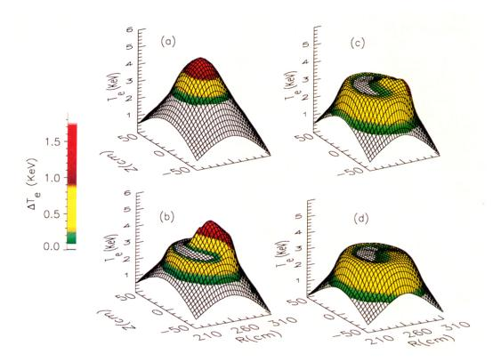
• Reconnection of the magnetic field in the plasma core drives the crash
