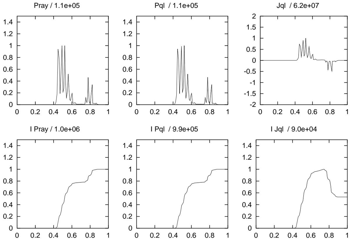
Power and current deposited *without diffusing* the current or the power. More rays would produce a smoother result. Horizontal axis is the square root of normalized poloidal flux.
