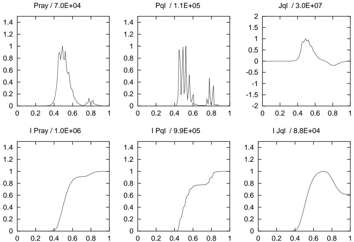
Power and current deposited *with diffusing* the current and then the power.
