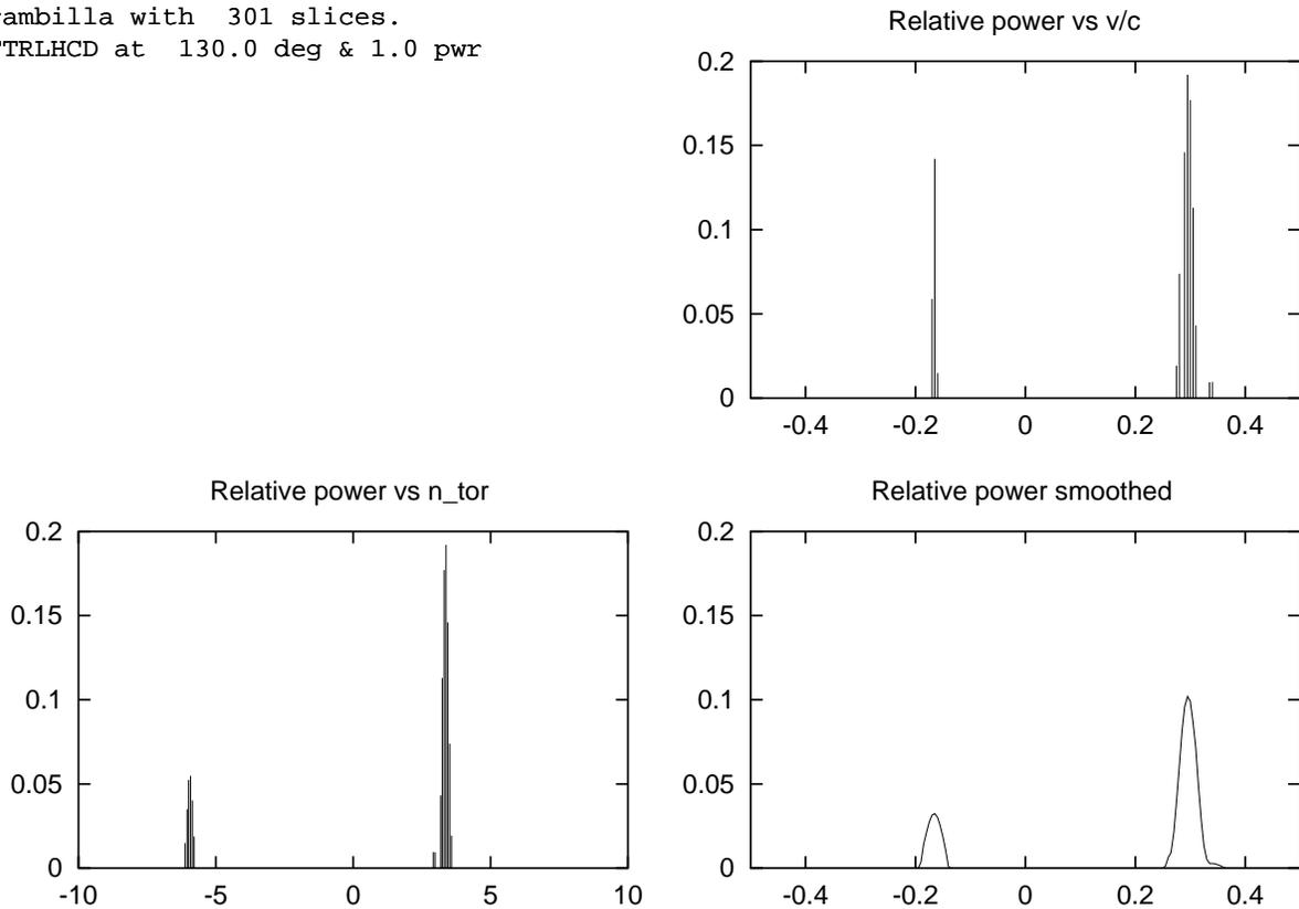
A launched spectrum from a Brambilla calculation, including the negative-going minor components.
