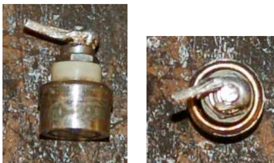
Figure 3: Bendix semiconductor-type, low breakdown voltage spark plugs.
