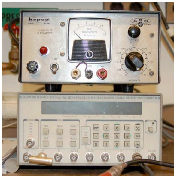
Figure 15: DDG (below). High voltage power supply (above).
