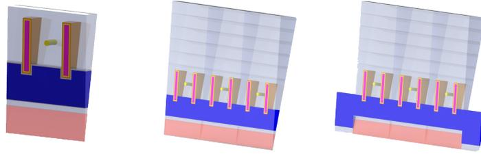
Figure 2: **Left:** Solid model of 10° solid model section of reactor. **Center:** Full-length solid model of 10° sector of reactor. **Right:** with end cap and axial ports; this model was the final model made for simulations
