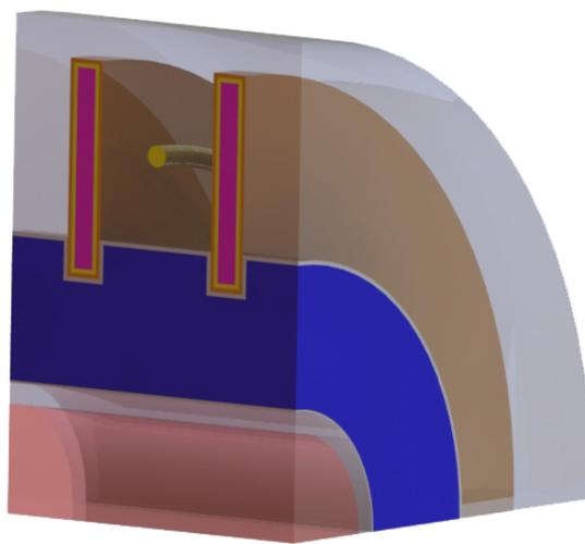
Figure 1: Initial solid model of reactor used for simulations. Model uses 90-degree symmetry of and model reactor as uniform, infinitely long cylinder.
