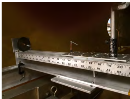
Figure 6: Translation stage. Potentiometer in back, with white marking.
