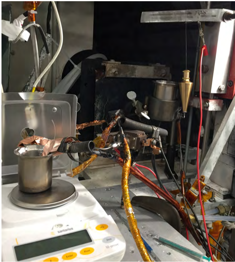
FIGURE 6: This is the full set up of the mass propellant feed system in the vacuum tank. It can be controlled via LabView and can be set to adjust the current and piston speed autonomously to achieve the desired flow rate. The heating coils around the pump are to keep the propellant in liquid state.
