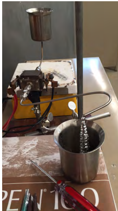
FIGURE 2: The JxB Pump set up, pumping gallium into a beaker.
