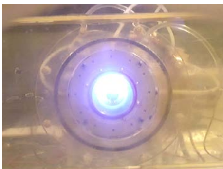
Figure 3: A current sheet produced during the firing of the MiGfPPT, captured from a frame of digital video.
