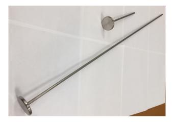
PPPL can provide electrodes on request. Dimensions are as follows: Material: Stainless steel Diameter: 1.9" Thickness: 1/4" Stainless rods: 1/4" diameter, grounded rod length =  $\sim$ 30"; HV rod length:  $\sim$ 8" Rods are threaded (you can also press fit) in the back of the disk
