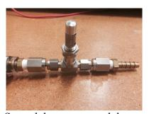
Swagelok www.swagelok.com Part # B-SS4 \$82 Brass Low-Flow Metering Valve, 1/4 in. Swagelok Tube Fitting
