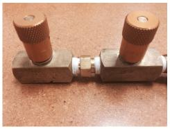
McMaster-Carr www.mcmaster.com # 46425K12 \$34.12 Easy-Set Needle Valve, Brass 1/4" NPTF
