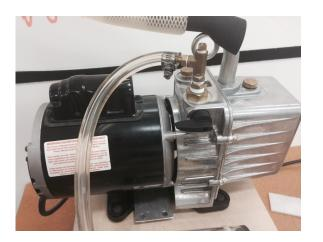
McMaster-Carr www.mcmaster.com Part # 4396K43 Rotary Vane Deep Vacuum Pump \$465.49
