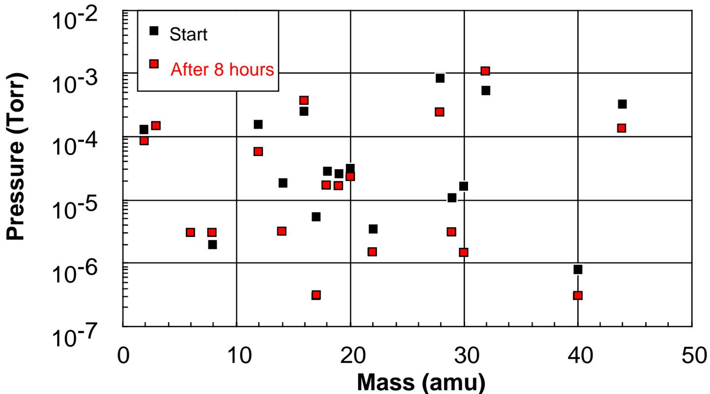
RGA spectra taken during He-O glow about 1/2 hour after the start and after about 8 hours of glow.
