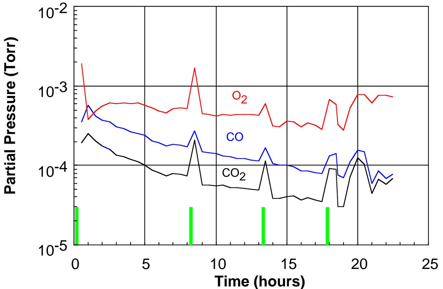
Partial pressures during He-O GDC. The data has been concatenated to remove the non-glow periods. The start times of the periods are indicated by green bars at the bottom of the graph.
