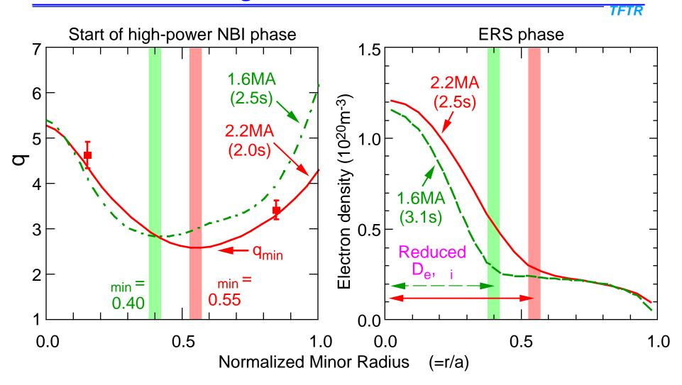
Location of transport barrier in ERS phase moves with min
