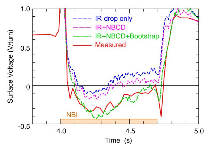
Negative surface voltage early in NB pulse with resistive model arises from flux-conserving changes in equilibrium during rise in plasma pressure
