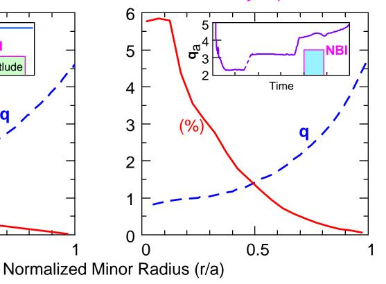
Both regimes have NBI fueling, low edge recycling, peaked profiles and T<sub>i</sub> > T<sub>e</sub>
