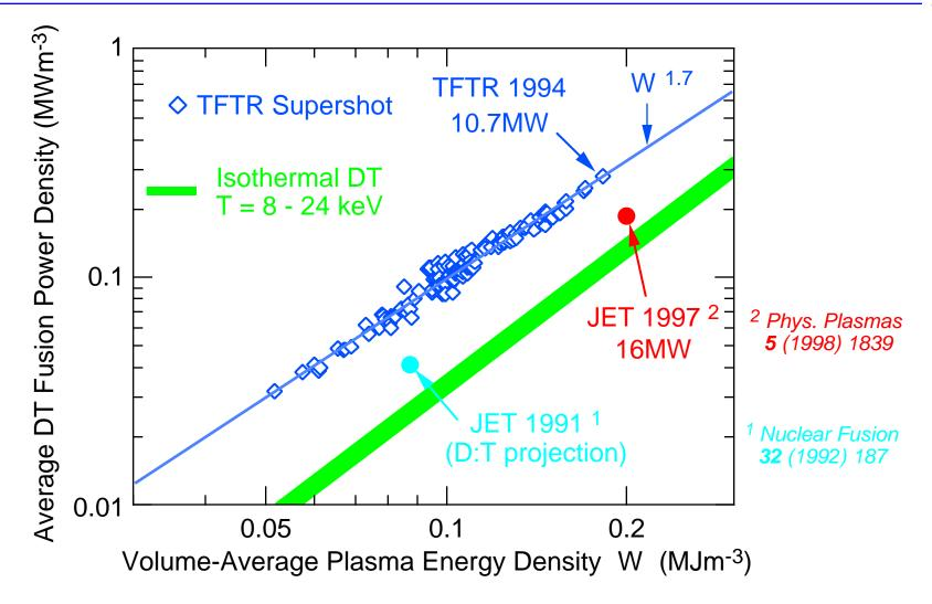
High reactivity allowed investigation of fusion alpha-particle physics in tokamak with moderate size and, therefore, confinement
