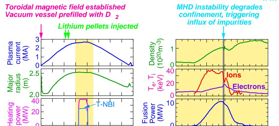
TFTR operated at or beyond original specifications in field, current, pulse length
