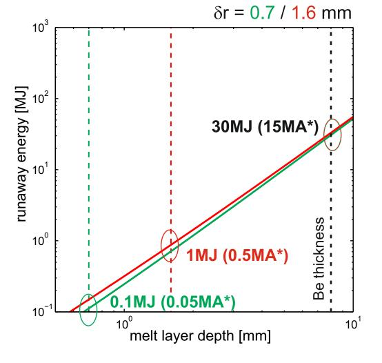
assume energy is deposited on timescale short compared to heat transport
