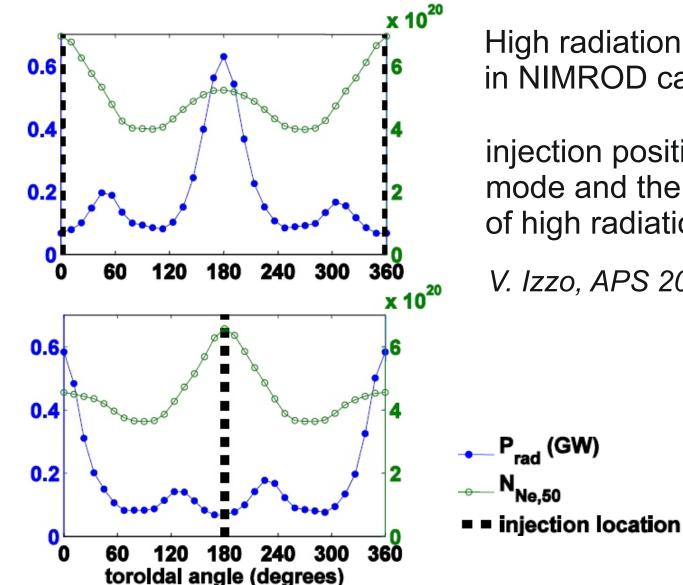
High radiation peaking observed in NIMROD calculations with TPF = 3.5
