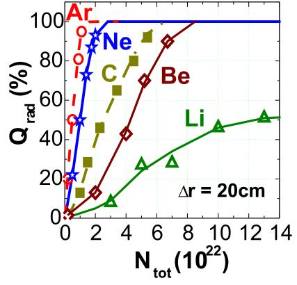
Dependence of radiated power fraction on impurity content at radiating layer of 20 cm width
