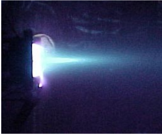
Fig. 8. Hall thruster operation
