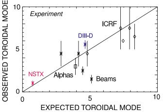
Most unstable mode number (larger amplitude at the edge) scales as  $n \sim a/q^2$ .
