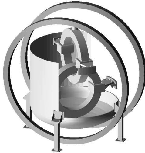
FIGURE 1. A cutaway drawing of CNT showing the vacuum vessel and the four circular coils.
