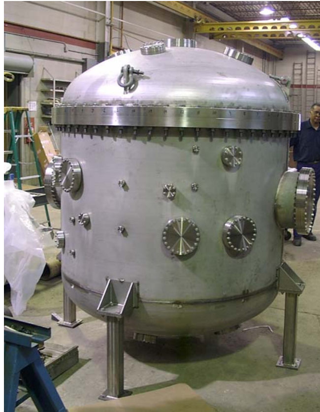
Figure 5. The CNT vacuum chamber complete after leak tests at Ability Engineering in South Holland, IL, USA
