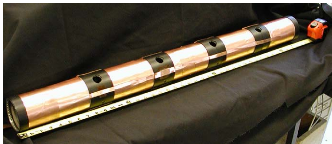
Fig. 2. The 1-m-long BaTiO 3 FEPS consists of 5 BaTiO 3 ferroelectric source segment individual sources with diagnostic ports between the sources.
