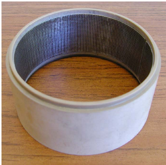
Fig. 1. Photograph of the 1.6"-long cylindrical BaTiO 3 ferroelectric segment.
