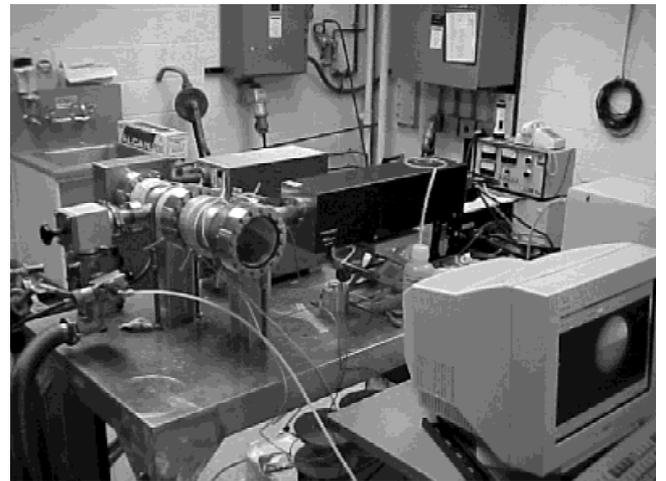
Fig. 1. Photograph of the ECR solenoid plasma source and the Langmuir probe.
