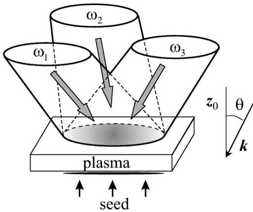
FIG. 1. Schematic of pump incident on plasma.
