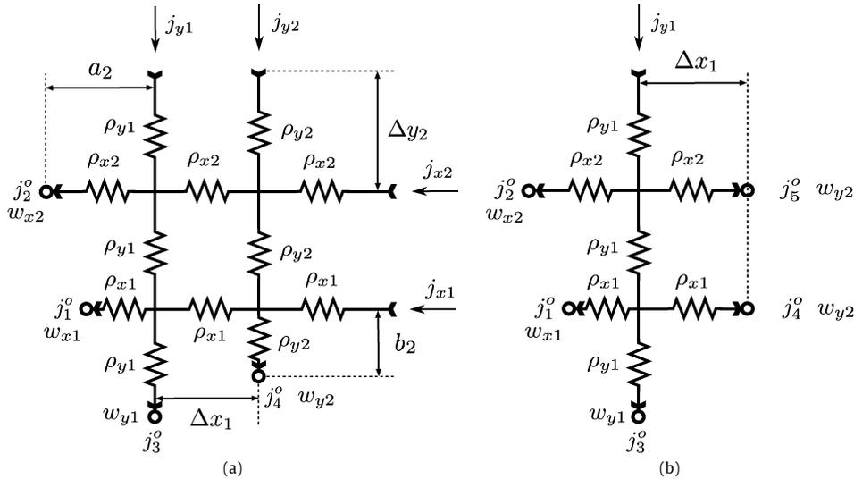
**Fig. 3.** (a) Electrical circuit equivalent to the simplest diffusion network formed by four intersecting diffusion paths. (b) The same circuit when the resistivity of the second vertical diffusion path is much smaller than all the others.
