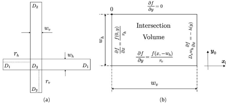
Fig. 5. (a) Two intersecting diffusion paths and their geometrical sizes; (b) intersection volume and the boundary conditions.
