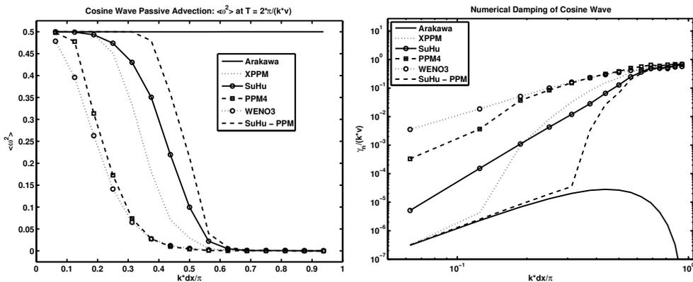
FIG. 4.3.  $\langle \omega^2 \rangle$  as a function of wave number for the passive advection of a cosine wave after one period  $T$  for the different algorithms (left), along with associated numerical damping factors  $\gamma_n$  (right) as defined by  $\langle \omega^2 \rangle(T) = \frac{1}{2} e^{-2\gamma_n T}$ .
