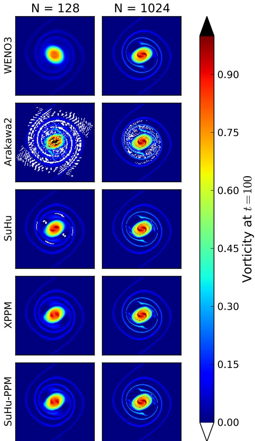
FIG. 4.4. Low ( $N = 128$ ) and high resolution ( $N = 1024$ ) vorticity solutions for the vortex merger problem with high Reynolds number  $Re = 10^5$  at  $t = 100$ , with the color scale spanning the minimum and maximum initial vorticity. Positivity violations appear white. Unphysical overshoots are black.
