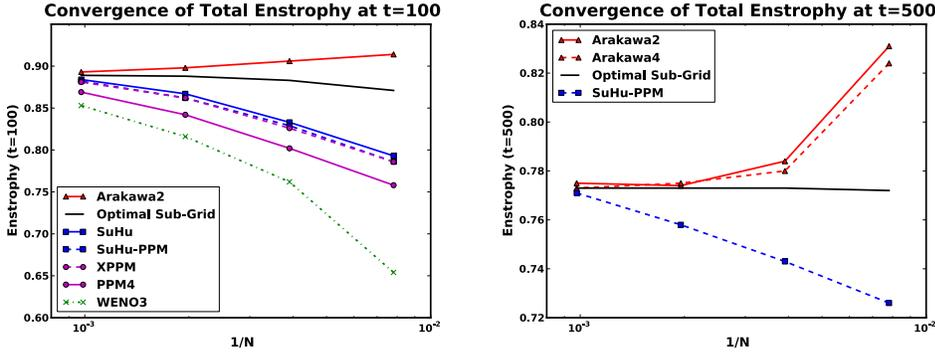
FIG. 4.6. Convergence of the total enstrophy at time  $t = 100$  (left) and time  $t = 500$  (right) vs.  $1/N$ , for grid sizes  $N = 128, 256, 512, 1024$ , for the high Reynolds number case. Also plotted are the solutions from an optimal sub-grid model.
