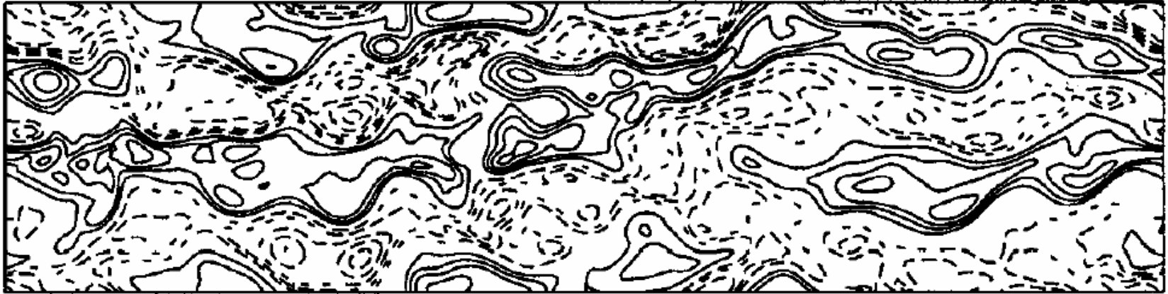
FIG. 2. Characteristic \phi contours in the outboard x - y plane. This snapshot was taken at the end of the ETG run shown in Fig. 1. The figure is 256\rho_e \times 64\rho_e .
