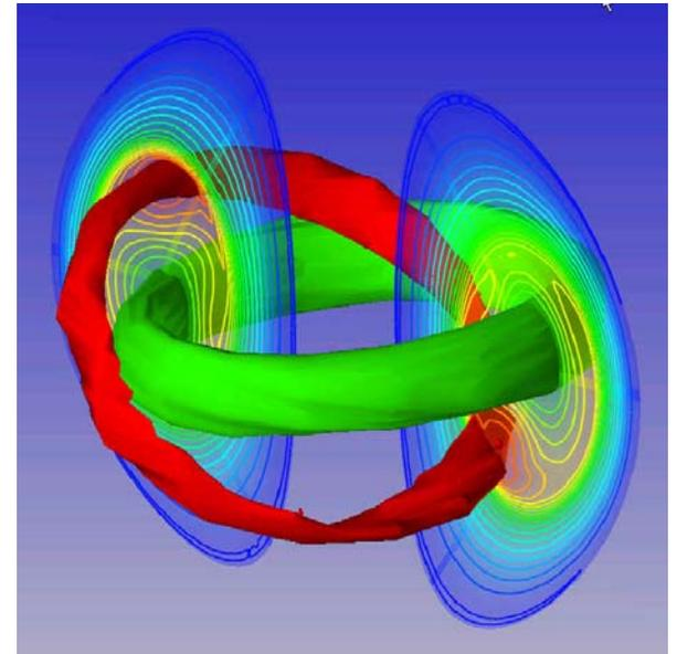
Evolution of pressure and magnetic topology from a NIMROD simulation of DIII-D
