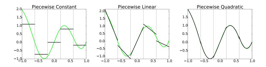
Standard finite-volume (FV) methods evolve just average value in each cell (piecewise constant), combined with interpolations
