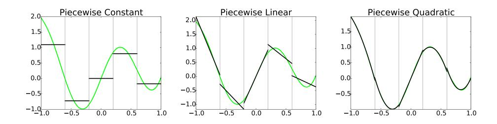
Don't get hung up on the word "discontinuous". Simplest DG is piecewise constant: equivalent to standard finite volume methods that evolve just cell averaged quantities. Can reconstruct smooth interpolations between adjacent cells when needed.
