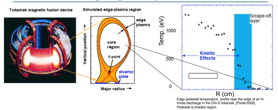
Present core gyrokinetic codes are highly optimized for core, need new codes to handle additional complications of edge region of tokamaks (& stellarators):
