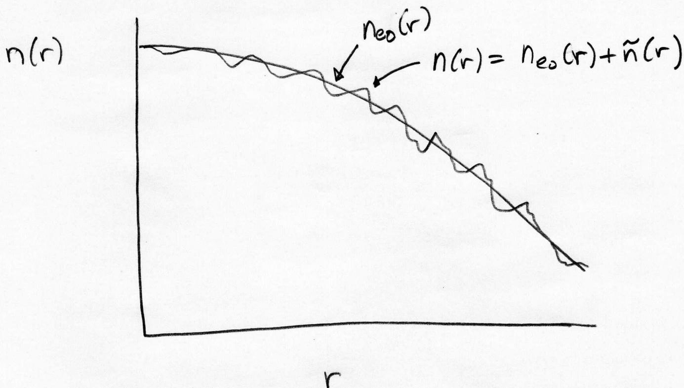
Instabilities driven by density (or temperature) gradients tend to saturate when  $\nabla \tilde{n}$  is large enough to offset  $\nabla n_0$  so the total density gradient vanishes at some places:
