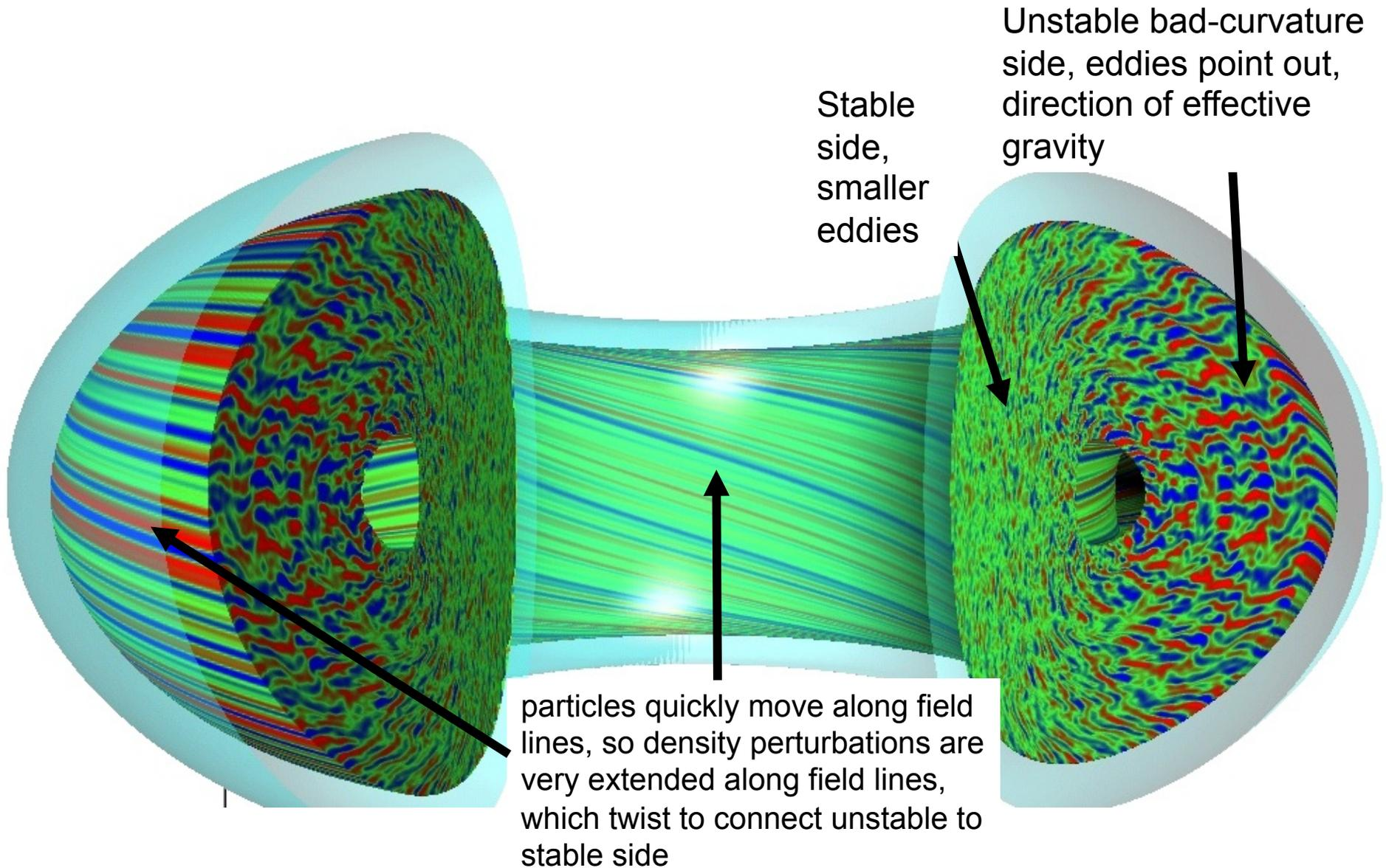
Note: plots such as on the last page make it look like there is extremely large turbulence in a tokamak. In fact, the relative density fluctuations are quite small,  $\tilde{n}/n_0 \sim 0.1\% - 1\%$  in the core region. What is being plotted on the last page are just the density fluctuations  $\tilde{n}(\mathbf{x})$ , because if we tried to plot contours of the total density  $n(\mathbf{x}) = n_0(r) + \tilde{n}(\mathbf{x})$ , you couldn't see the small amplitude fluctuations (see below).
