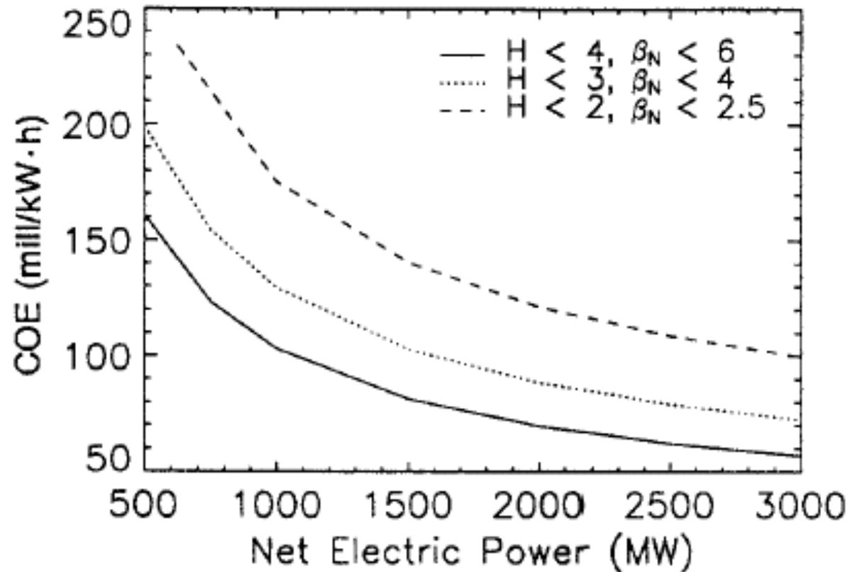
Improved confinement factor  $H$  helps even in very large reactor-scale devices. (Have to increase  $H$  &  $\beta$  together.)
