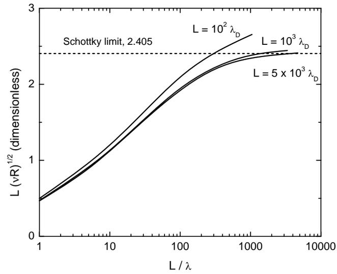
Fig. 4. The collisional plasma-sheath model approaches the Schottky limit for strong collisionality and large plasmas. The calculations are done for cylindrical geometry, proportional ionization, and  $T_i/T_e = 0.1$ .
