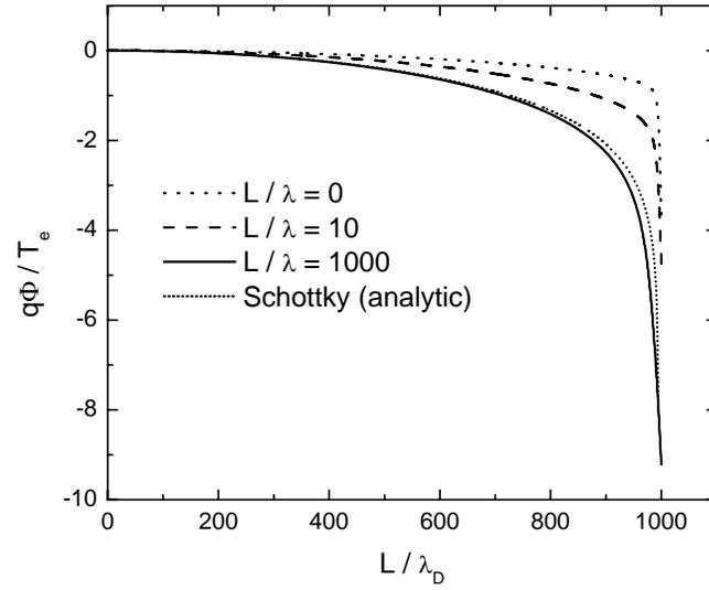
Fig. 3. The change of the potential profile with increasing collisinality. The calculations are for cylindrical geometry, proportional ionization, plasma dimension  $L = 1000\lambda_D$ , ion temperature  $T_i/T_e = 0.1$  and various mean free paths. The short-dotted line is the analytic result from the Schottky theory. The curves end at the potential of the wall.
