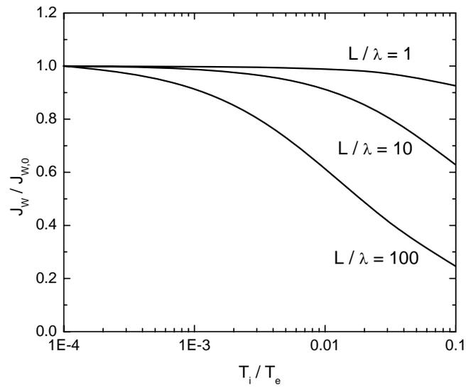
Fig. 2. The decrease of the ion flux to the wall with increasing ion temperature. The calculations are for plasma size  $L = 1000\lambda_D$ , planar geometry and ionization proportional to the electron density. The three curves are for different collisionality of the plasma.
