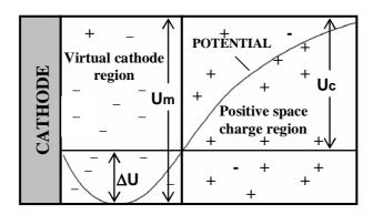
Fig.8. Schematic presentation of the virtual cathode structure for a refractory cathode material.
