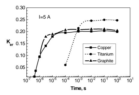
Fig.4b. Time dependence of the cathode evaporation fraction.
