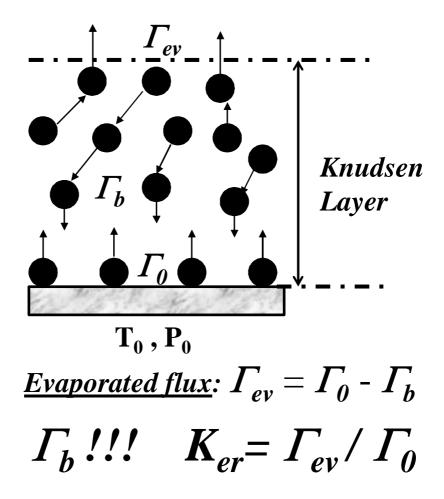
Fig.1 Schematic diagram of rare atomic collisions in the Knudsen layer. The back flux  $\Gamma_b$  to the surface is generated at the length of Knudsen layer and  $\Gamma_0$  is the direct atom flux in accordance with target temperature  $T_0$  and saturated vapor pressure  $P_0$ .
