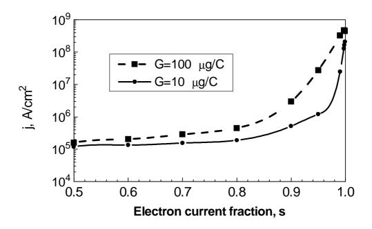
Fig.10. Spot current density as function on electron current fraction in the spot with cathode erosion rate as parameter.
