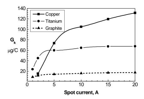
Fig.6a. Steady state cathode erosion rates normalized by the spot current as functions of the spot current.
