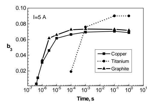
Fig.5b. Time dependence of the normalized plasma velocity at the external boundary of the Knudsen layer.
