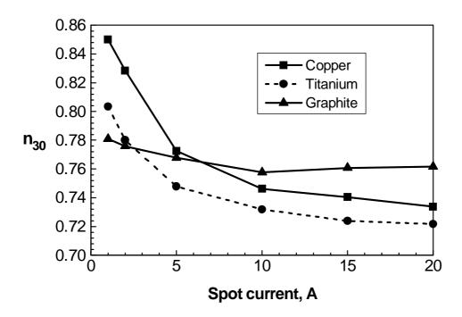
Fig.7a. Heavy particle densities at the external boundary of the Knudsen layer  $n_3$  normalized by the saturated density  $n_0$  as functions of the spot current.
