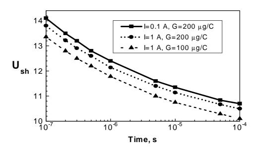
Fig. 13. Time dependence of the sheath potential drop for a *Hg* cathode.
