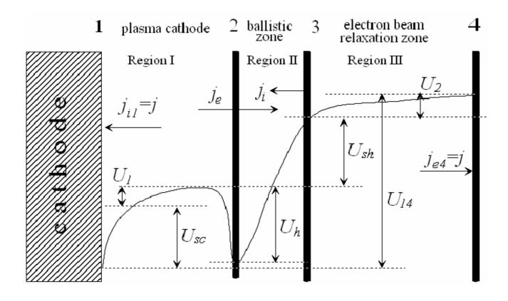
Fig.12. Near cathode (mercury) schematic potential distribution in the cathode plasma region I (screening potential drop  $U_{sc}$ ), in double sheath  $U_{sh}$  (region II) and in the electron beam relaxation zone (region III).  $U_1$  and  $U_2$  is the potential drop in the plasma regions I and III respectively.
