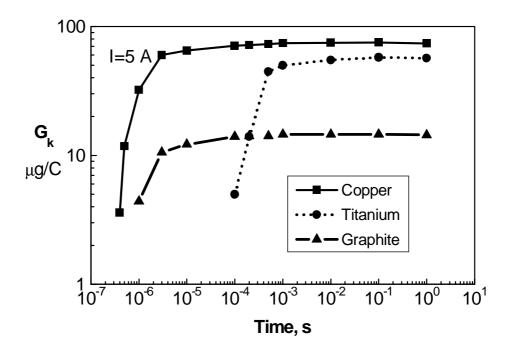
Fig.6b. Time dependence of the cathode erosion rates normalized by the spot current.
