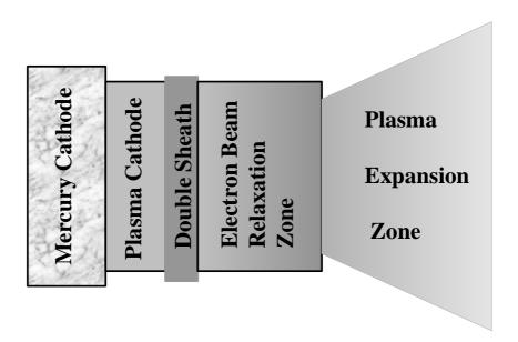
Fig.11. The plasma layer structure with a plasma cathode and an electron beam relaxation zone near a Hg cathode.
