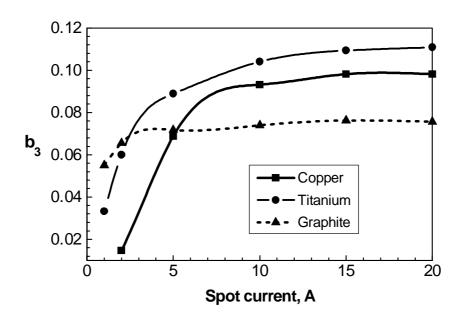
Fig.5a. Steady state normalized plasma velocity at the external boundary of the Knudsen layer as functions of the spot current.
