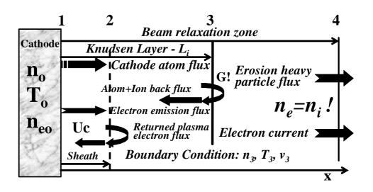
Fig.3. Model of vacuum arc cathode evaporation. Structure of kinetic layers in the cathode current-carrying plasma.
