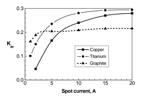
Fig.4a. Steady state cathode evaporation fraction as functions of spot current.
