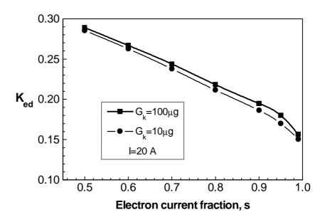
Fig.9. Electric field at the sheath-plasma interface normalized by the ratio of the electron temperature to the Debye length as a function of the electron current fraction in the spot with W cathode erosion rate as parameter.
