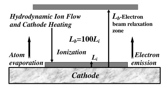
Fig.2. Schematic model of the electron beam relaxation zone  $L_b$  and ion mean free path  $L_i$  in a vacuum arc cathode region illustrating the relative lengths and showing the ion flux to the cathode which can be calculated by hydrodynamic treatment of the ion flow.
