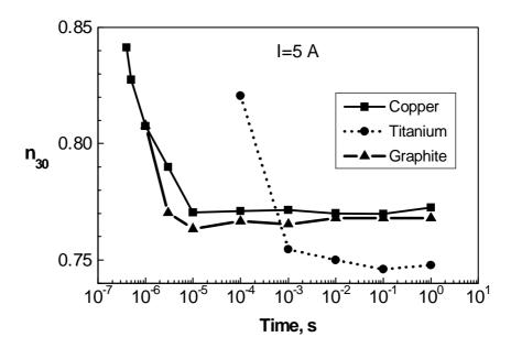
Fig.7b. Time dependence of heavy particle densities at the external boundary of the Knudsen layer  $n_3$  normalized by the saturated density  $n_0$ .
