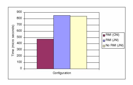
In CNI, Java classes are C++ classes (but not the other way around). The entire application (C++ and Java) is compiled to an executable, making access faster than through JNI.
