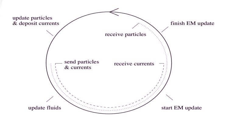
Overlapping communication (dashed lines) and computation (solid line) is one of the reasons VORPAL simulations scale to many processors
