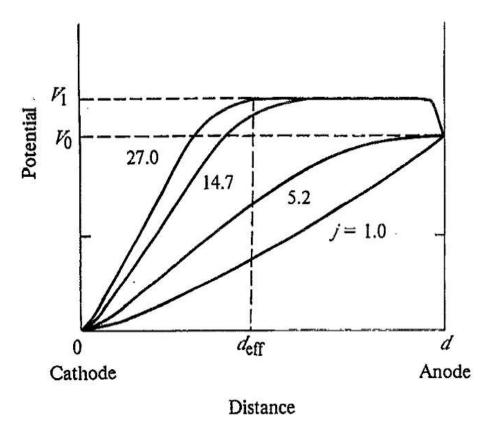
The potential in the simulations develops similarly to the predictions by the theory of Kozyrev et al., providing more confidence in the simulation results
