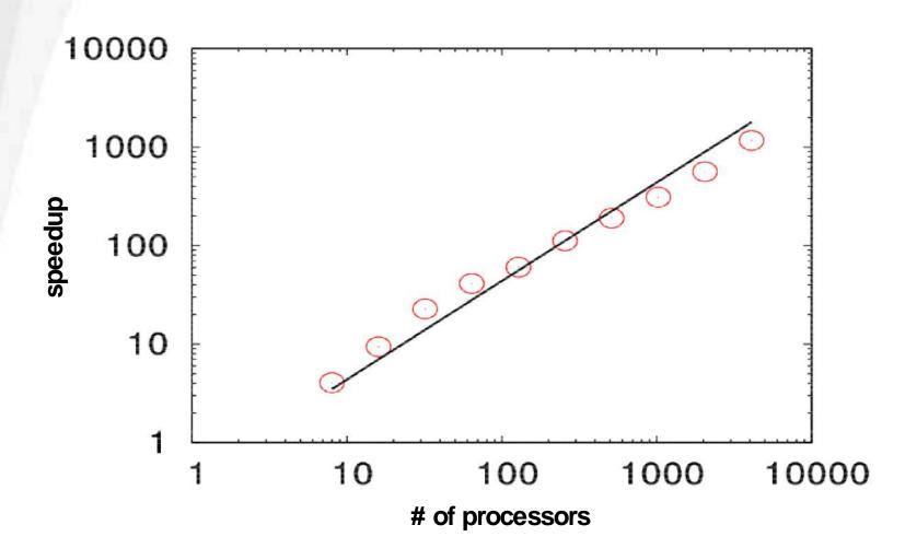
Simulations of laser-plasma interaction performed at NERSC show near-linear speedup to 4000 processors
