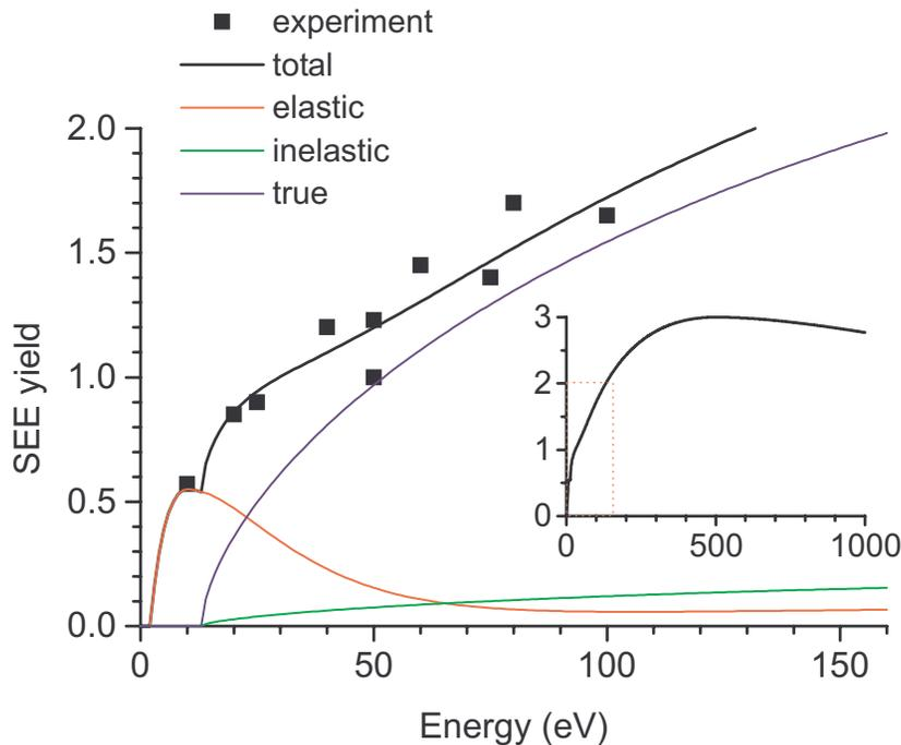
The SEE coefficient (ratio of emitted and incident electron currents) versus the energy of incident electrons.
