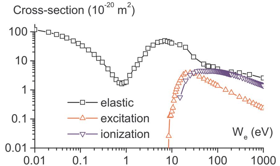
Cross-sections of different electron-neutral collisions versus the electron energy.
