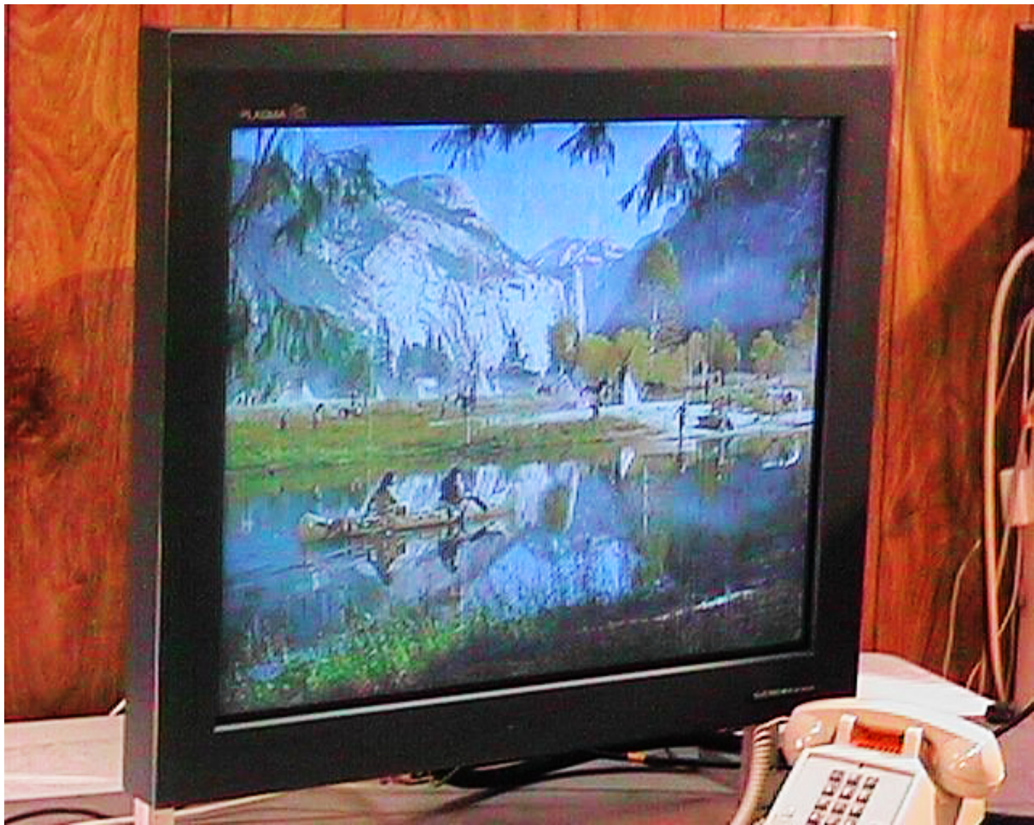
EPI prototype color AC PDP - 30 inch (diagonal)
