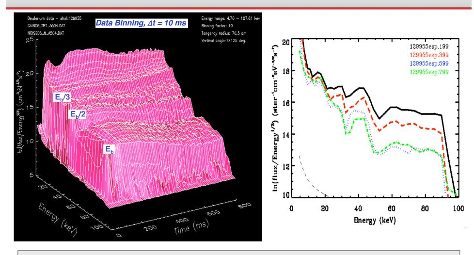
• Depletion of the NPA spectrum in the range  $E_b/2 \le E \le E_b$  by ~ 3 e-foldings is due to the combined effects of  $n_e$  ramp-up and MHD-induced energetic ion redistribution.
