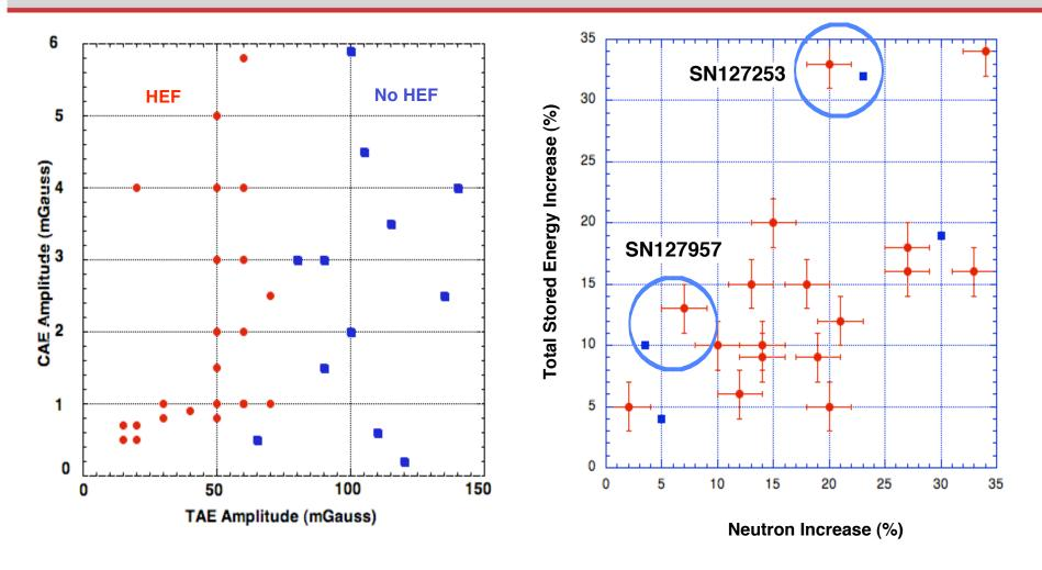
• The experimental neutron rate and total stored energy increase during the HEF (right plot). Similar increases are observed in some TRANSP analyses (blue circles).
