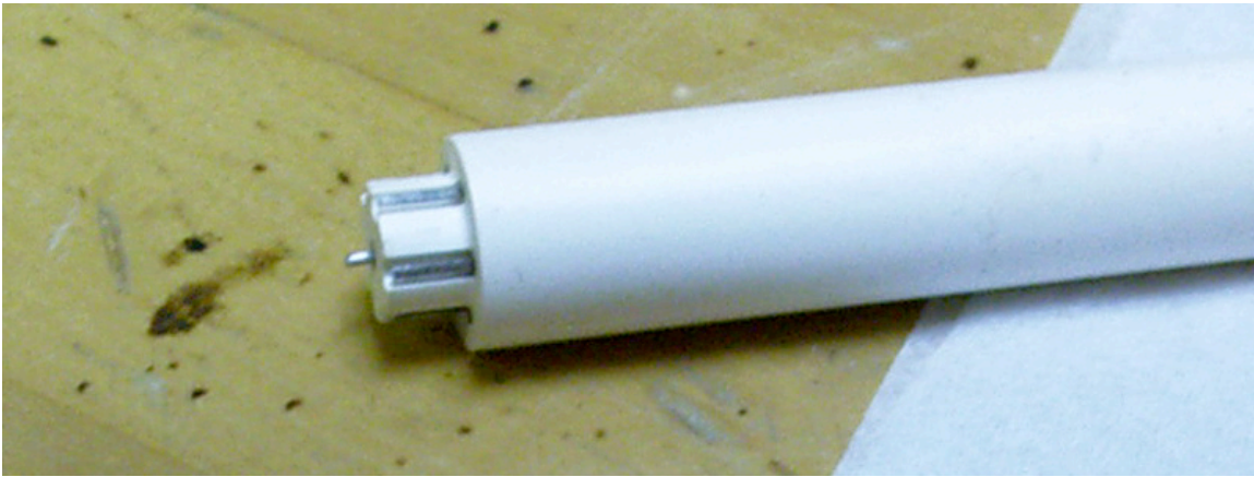
Figure 2.5: Photograph of HSX Mach probe. Note the outward facing tips used for the flow measurements (two are easily visible) and the proud pin used for measuring the floating potential. The tips are made of tungsten and the white body of the probe is boron nitride.
