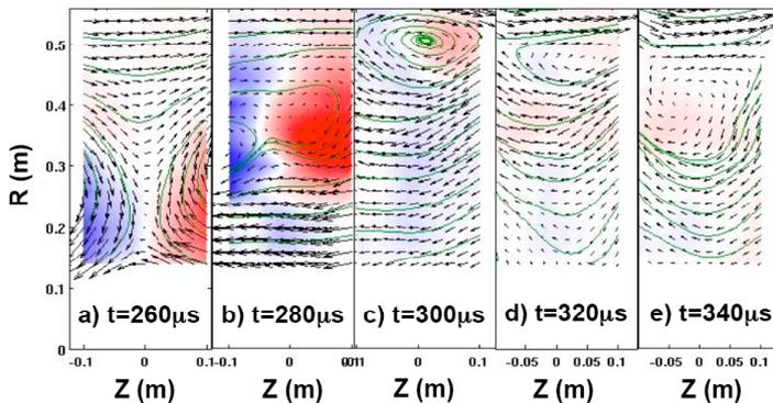
FIG. 6. Shifting motion for a large mirror ratio discharge without the center-column. The plasma shifts outward and back at the angle of the 90-channel probe, on a time-scale shorter than the discharge lifetime.
