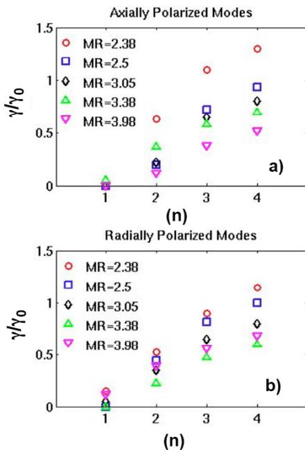
FIG. 11. Linear Growth rates of low- $n$  co-interchange modes (axial and radial polarizations) for FRCs with different mirror ratios.
