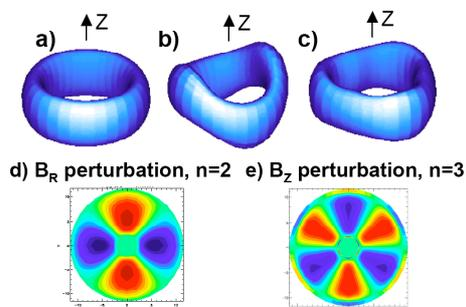
FIG. 1. a) Unperturbed pressure isosurface, isosurface after b) an axially polarized  $n=2$  mode, and c) a radially polarized  $n=3$  mode. Also shown are d) the midplane  $B_R$  perturbation for the axially polarized  $n=2$  mode and e) the midplane  $B_z$  perturbation for the radially polarized  $n=3$  mode.
