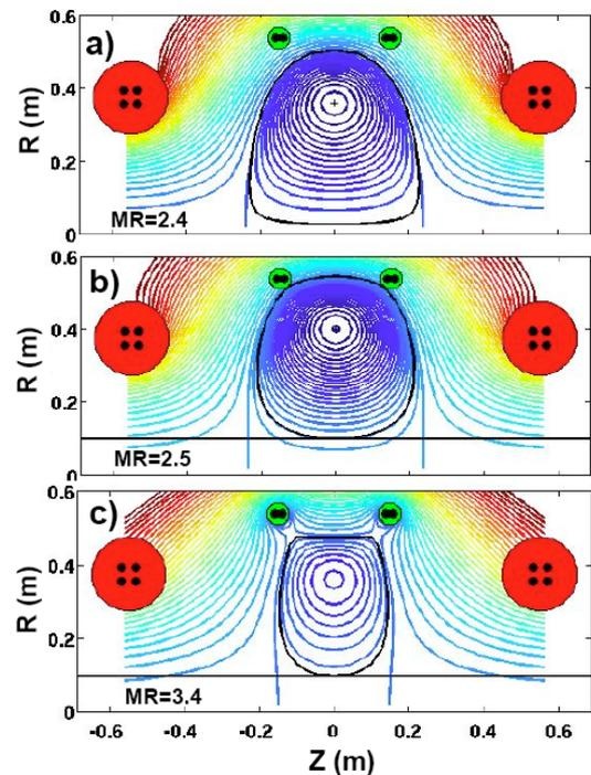
FIG. 8. Poloidal flux contours from example equilibria for three different FRCs in MRX.
