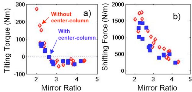
FIG. 10. Tilting torque and shifting force, normalized to the small tilt and displacement, respectively, as a function of the mirror ratio.
