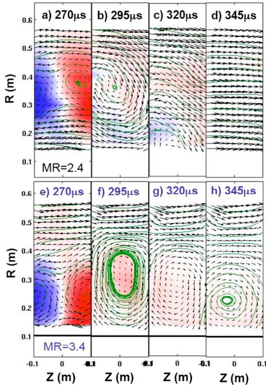
FIG. 3. (a-d) Four images of the time evolution of a discharge which develops a large  $n=1$  tilt mode (no center-column,  $MR=2.4$ ), and (e-h) four similar images from a very oblate plasma with a center-column ( $MR=3.4$ ), which displays more robust stability. Some streamlines (green, not flux lines) are illustrated to guide the eye. Colors represent toroidal fields from  $-0.5$  to  $0.5$  Tesla, with red positive.
