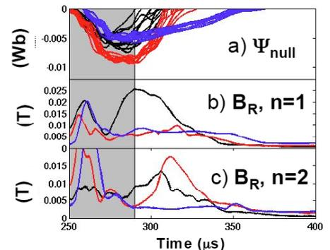
FIG. 4. Time evolution of (a) the poloidal flux at the field null, (b) the  $B_R$ ,  $n=1$  perturbation, and (c) the  $B_R$ ,  $n=2$  perturbation.
