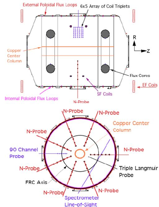
FIG. 2. (top) Side-view of MRX showing flux-cores, SF & EF coils, center-column, and the 90-channel probe array. (bottom) End-on view of MRX illustrating the N-probe array.
