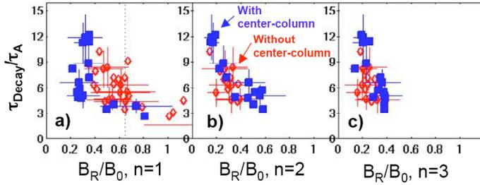
FIG. 7, Dependence of the plasma decay-time on the normalized  $B_R$  perturbations. The points on the right of the dotted line in (a) are not plotted in (b) and (c). Red, open (blue, closed) symbols correspond to discharges without (with) the center-column.
