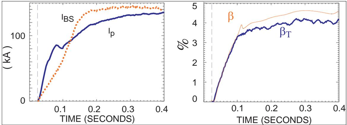
FIG. 5. Waveforms from time-dependent simulation of high-beta NCSX discharge. (a) Plasma current (programmed) and calculated bootstrap current. (b) Calculated beta values using tokamak ( $\beta_T$ ) and stellarator ( $\beta$ ) definitions.
