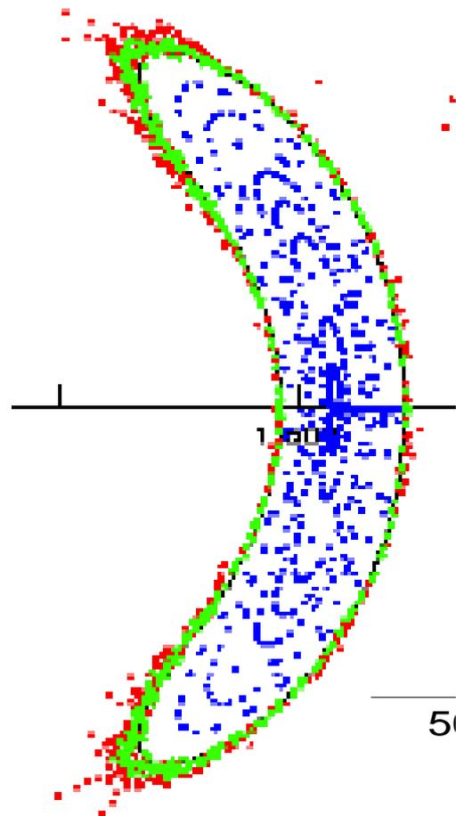
FIG. 7 Poincaré plots of scrapeoff field lines started at the inboard and outboard midplane within 0-1 cm of the nominal (VMEC) boundary and followed for 20 toroidal revolutions.
