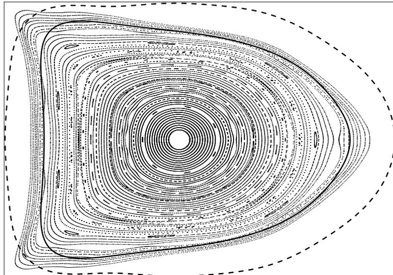
FIG. 2. Poincaré plots of PIES magnetic surfaces for target free-boundary PIES equilibrium at  $\beta=4.1\%$  for finite-cross section model of NCSX coils. Dashed line: first wall; solid line: VMEC equilibrium boundary.
