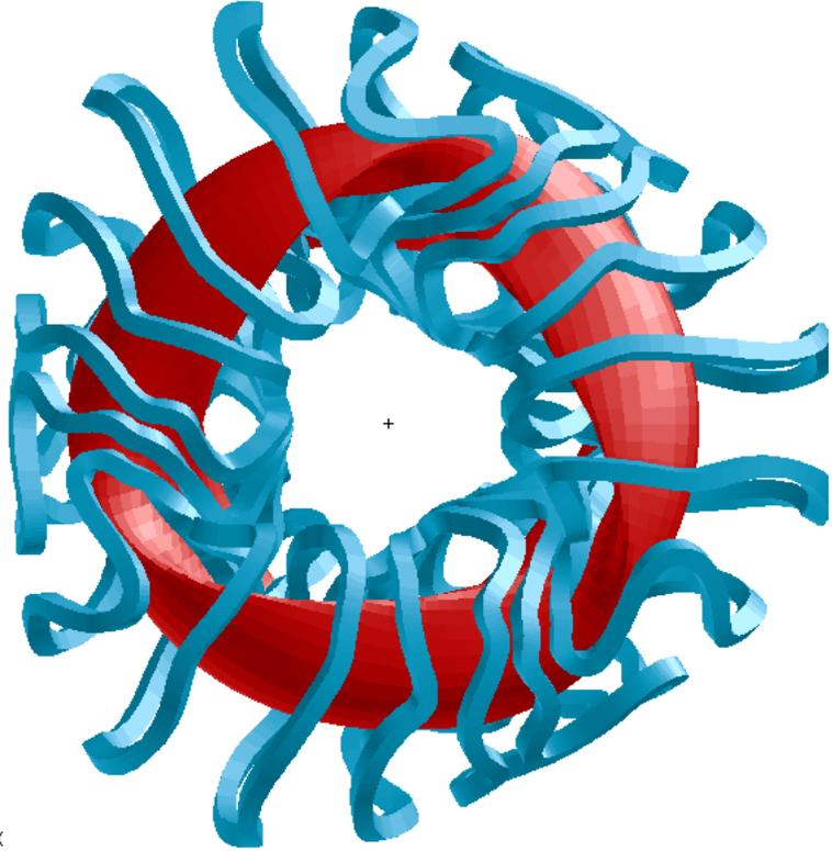
FIG. 1. NCSX modular coils and reference plasma. The coil system also includes toroidal, poloidal, and helical-field trim coils, not shown in the figure.
