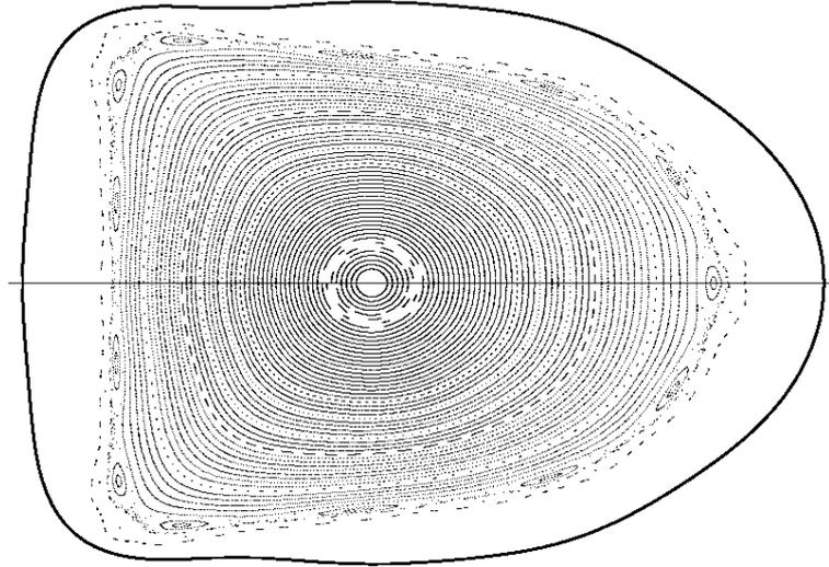
FIG. 3. Poincaré plots of PIES magnetic surfaces for vacuum configuration with iota of 0.43-0.46 (filamentary coil model). Dashed line: first wall boundary.
