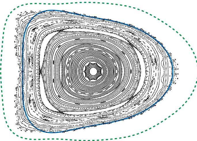
FIG. 6. Poincaré plots of PIES magnetic surfaces for equilibrium at  $t = 303$  ms in discharge simulation.
