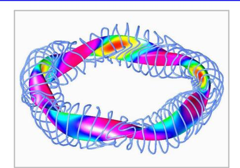
Confine a plasma of temperature 10<sup>8</sup>C by making magnetic field lines wrap around a toroid, the charged particles in the plasma follow the field lines and are confined.
