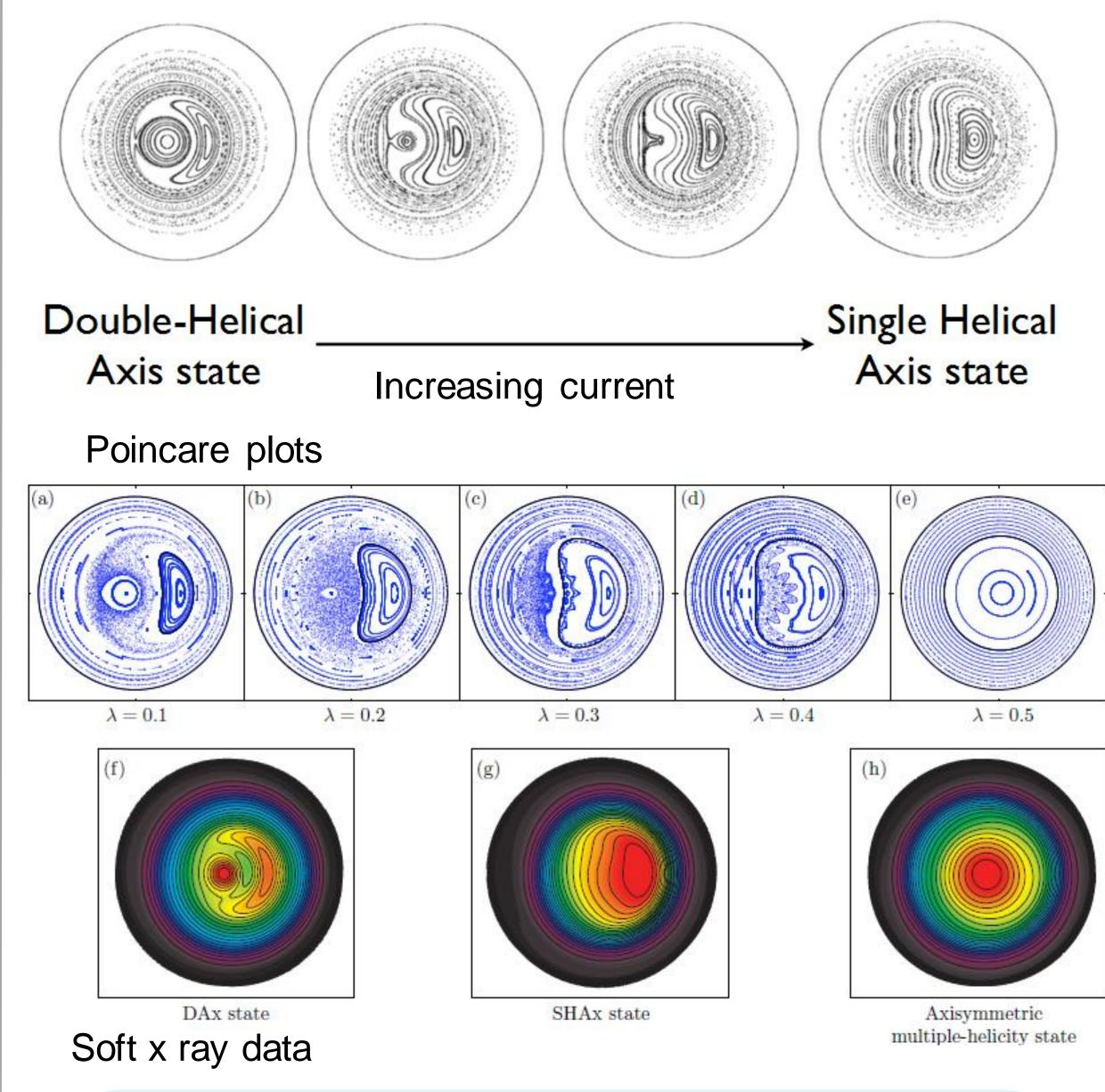
Ideal MHD (with assumed nested flux surfaces) cannot model the Double-Helical Axis state. [1] P. Martin et al., Nuclear Fusion 49, 104019 (2009).
