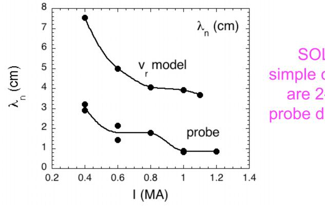
SOL widths from simple convective model are 2-3 x larger than probe density SOL width
