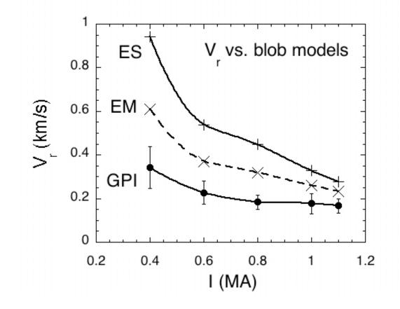
simple blob model velocities are 2-3 x larger than GPI convective speed
