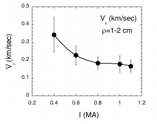
Ohmic current scan (#1090813005-020) I=0.4 - 1.1 MA B= 2.3 - 6.0 T q(95) = 3.7  $<n>=0.8 - 1.6 \times 10^{14} \text{ cm}^{-3}$   $n (\rho=1.5 \text{ cm}) \sim 1 \times 10^{13} \text{ cm}^{-3}$  $T_e (\rho=1.5 \text{ cm}) \sim 20 \text{ eV}$
