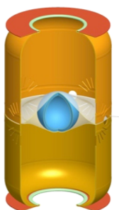
Fig. 58: Target suspended by the “tent” within the hohlraum.
